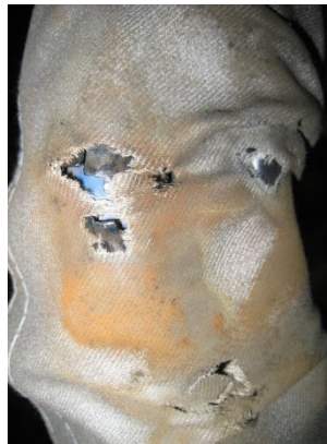
Fig. 7.2.3 (b) Damage on the cable protective sleeve
