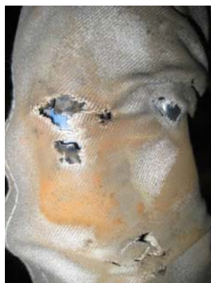
Fig. 7.2.2 (b) Damages on the cable protection sheath
