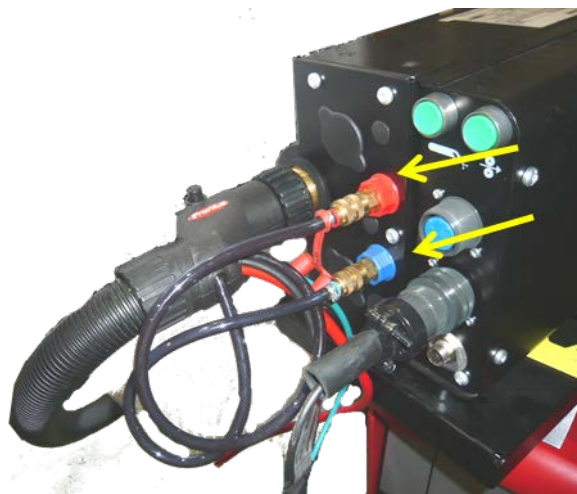
Fig. 2.2.4 (f) Connection of water cooling hose between the feeder and the hose pack
