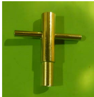
Fig. 7.6.1 (a) Special fixture for removing the torch neck
