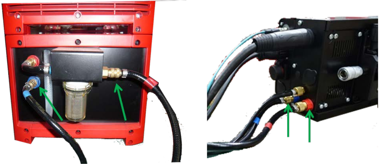
Fig. 2.2.4 (e) Connection of the water cooling hose between water cooling unit and the feeder
