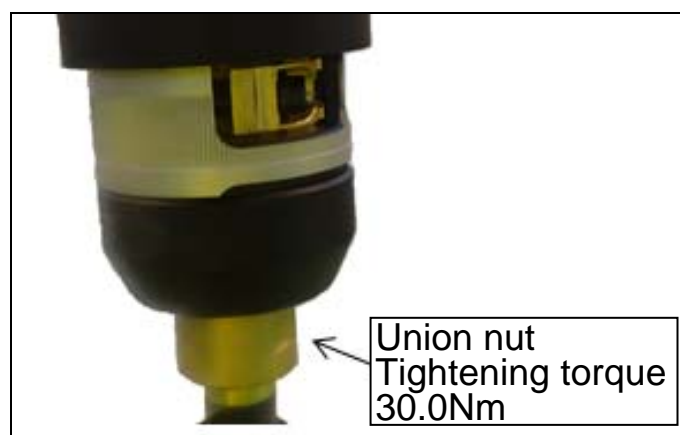
Fig. 6.2 Check of the union nut
