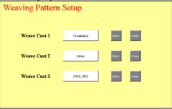
Press the Edit button of the weaving pattern you want to set up. Press the Demo button when if want to see the weaving pattern which have already been set.
