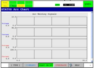
3 Execute TP Program with welding. The time chart graphs of command and feedback values between Arc Start and Arc End instruction are automatically traced. The actual output value is displayed by the numerical values under the output signal name of each graph.
