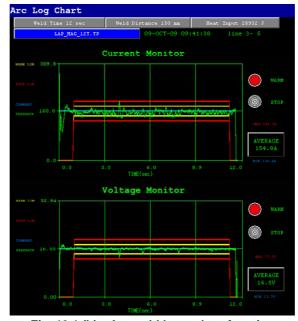
Fig. 19.1 (b) Arc weld log – chart function
