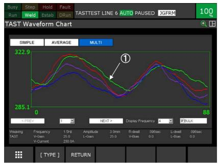
Fig. 20.6.4(e) Simultaneous single cycle display mode screen
