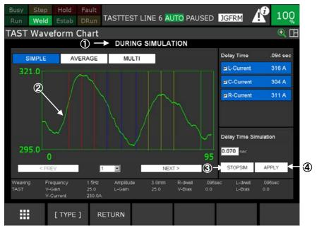
Fig. 20.6.4(b) Delay time simulation mode screen
