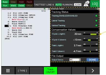
Displays each compensation value during tracking in real time.
