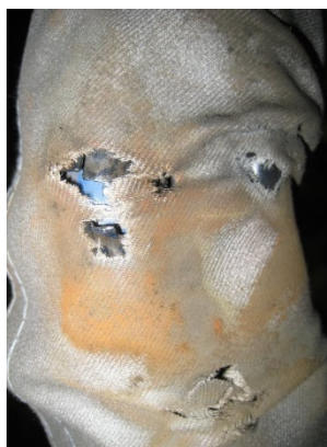
Fig. 2.2.3 (b) Damage on the cable protective sleeve
