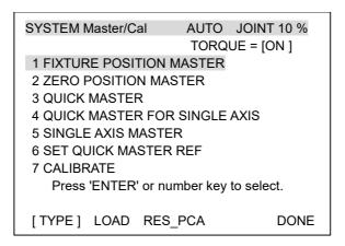
2 Select [4 QUICK MASTER FOR SINGLE AXIS]. The quick master for single axis screen will be displayed.
