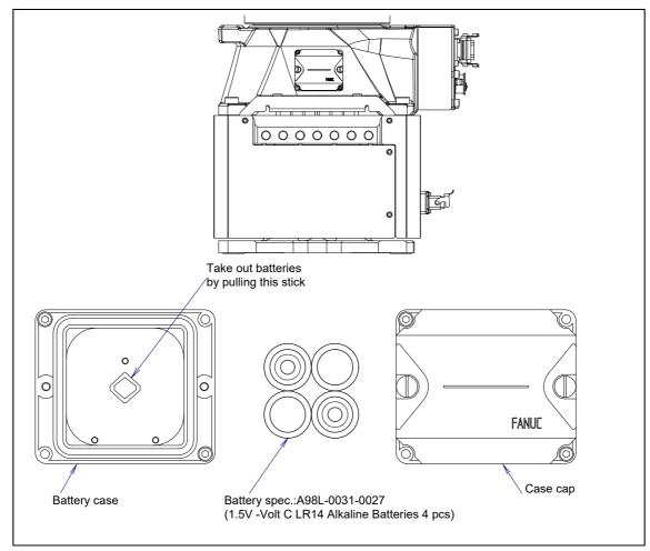
Fig. 7.3.1 (a) Replacing the battery
