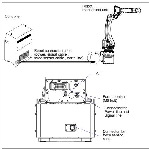
Fig. 2 (a) Cable connection
