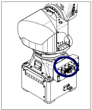
Fig. 7.2.3 (b) Connector Inspection points
