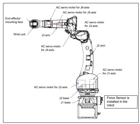
Fig. 3.1 (a) Mechanical unit configuration
