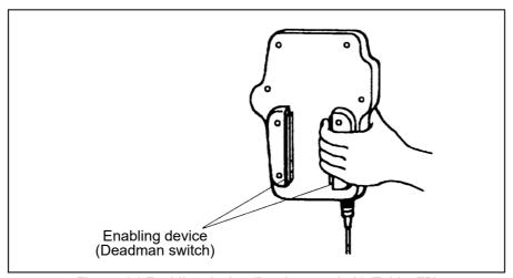
Fig. 4.4 (a) Enabling device (Deadman switch) (Tablet TP)
