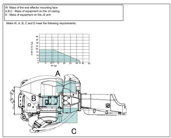
Fig. 4.2 (a) Loading condition
