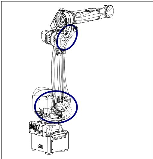
Fig. 7.2.3 (a) Inspection points of the mechanical unit cables
