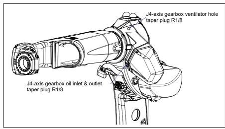
Fig. 7.3.2.3 (a) Greasing point of J4-axis gearbox
