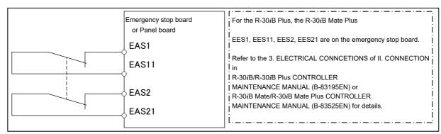
Fig. 2.4.2 (b) Connection diagram for the signal of the safety fence
