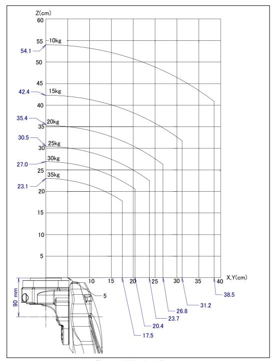
Fig. 3.4 (a) Wrist load diagram
