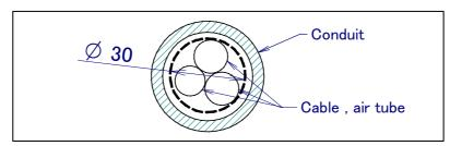
Fig. 10.1 (b) Diameter of cable and air tube in conduit
