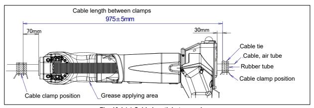
Fig. 10.1 (a) Cable length between clamp
