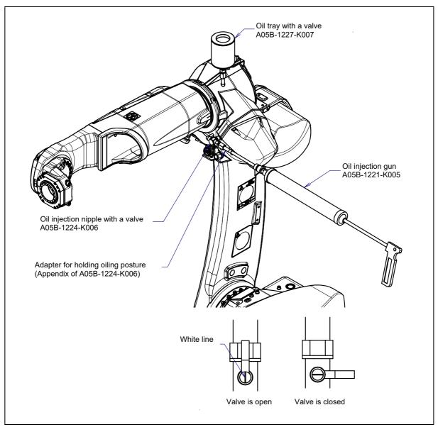
Fig. 7.3.2.3 (b) Oil injection by oil gun (oiling of J4-axis gearbox)
