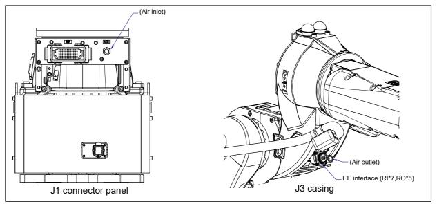
Fig. 5.3 (b) Interface for option cable (A05B-1228-H621#12 is specified)
