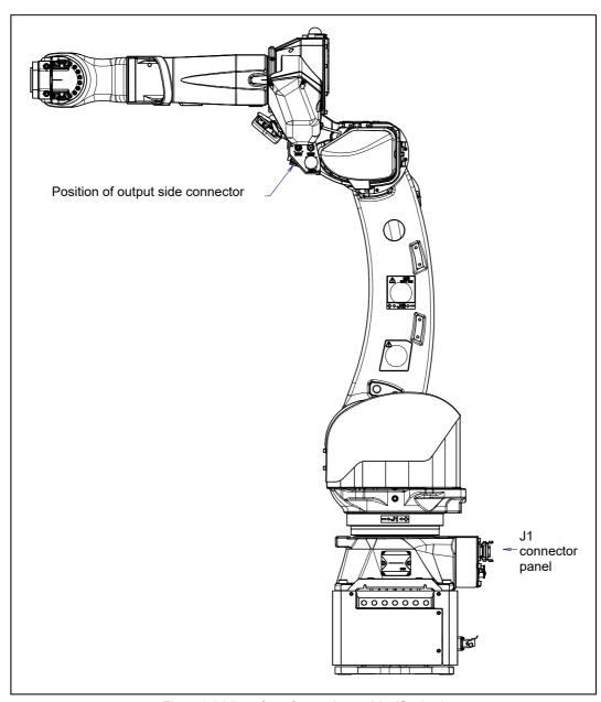
Fig. 5.3 (a) Interface for option cable (Option)
