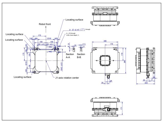
Fig. 1.2 (a) Dimensions of the robot base
