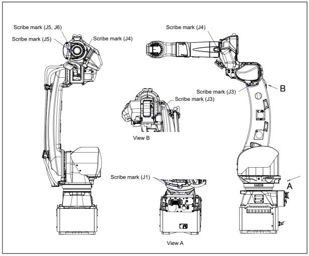
Fig. 8.3 (a) Zero-position mark (witness mark) for each axis
