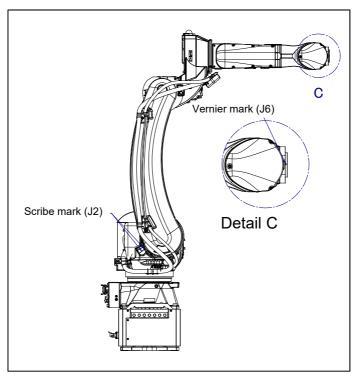
Fig. 8.3 (b) Zero-position mark (witness mark) for each axis
