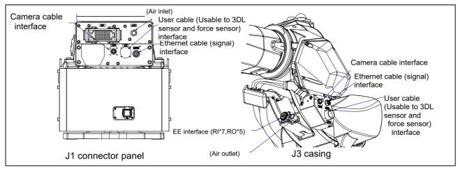
Fig. 5.3 (c) Interface for option cable (A05B-1228-H622#12 is specified)
