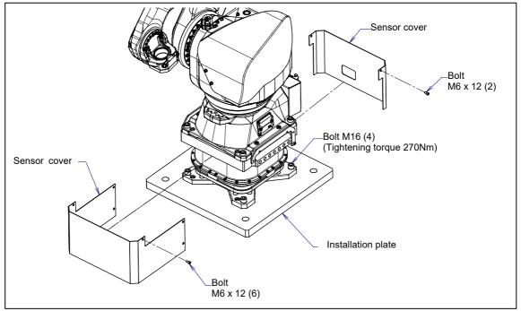
Fig. 1.2.1 (e) Robot installation
