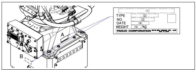
Position of label indicating mechanical unit and force sensor specification number
