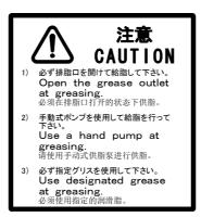
Fig. 5.11 (a) Greasing and degreasing label
