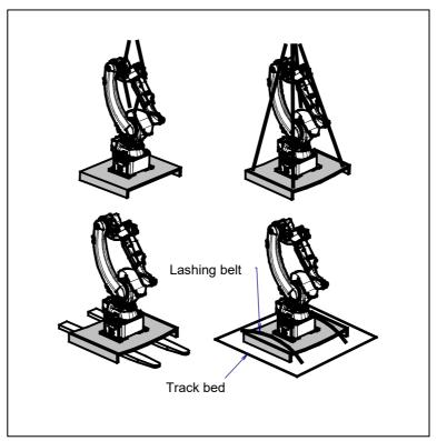
Fig. 1.1 (e) Wrong robot shipment status
