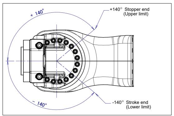
Fig. 3.3 (e) J5-axis motion limit
