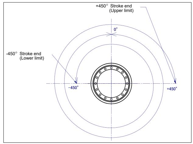
Fig. 3.3 (f) J6-axis motion limit
