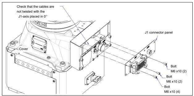
Fig. 8.1 (a) Confirming the state of cable (J1-axis)
