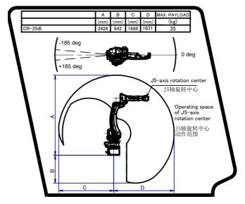
Fig. 5.11 (f) Operating space and payload label
