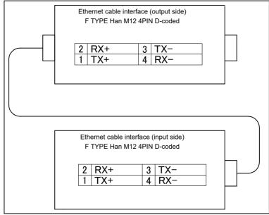
Fig. 5.3 (f) Pin layout for Ethernet (ES) cable interface (option)
