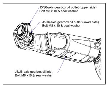
Fig. 7.3.2.4 (a) Oil inlet and outlet
