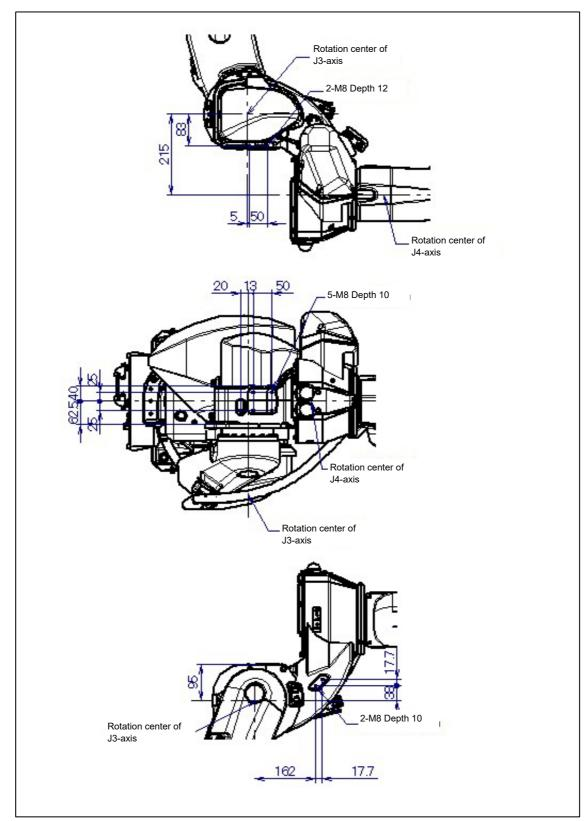
Fig. 4.2 (b) Equipment mounting faces (1/2) (A+B+C part)
