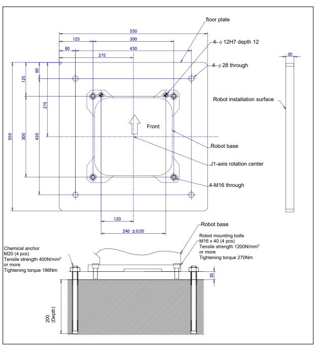
Fig. 1.2.1 (f) Example of installing the robot
