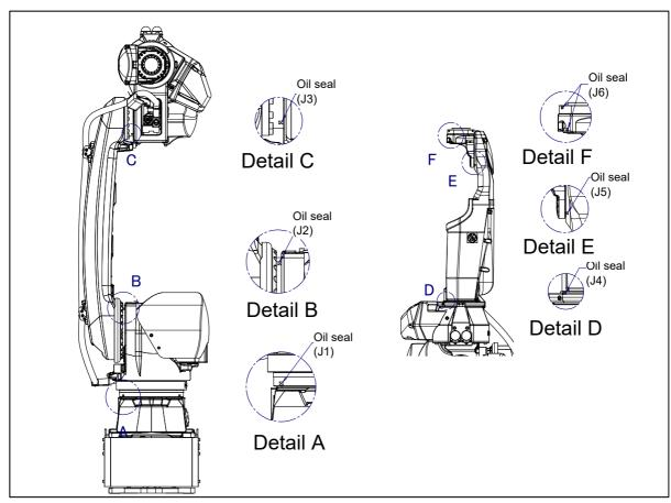
Fig. 7.2.1 (a) Check parts of oil seepage
