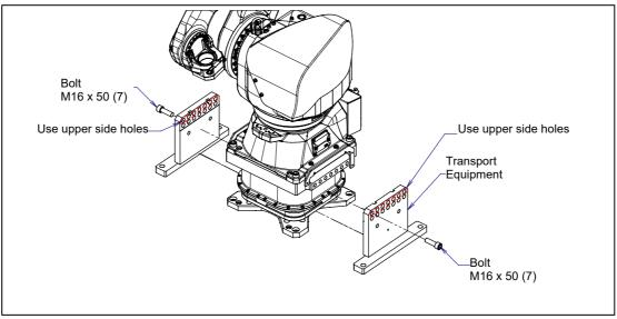
Fig. 1.2.1 (c) Removing the transport equipment
