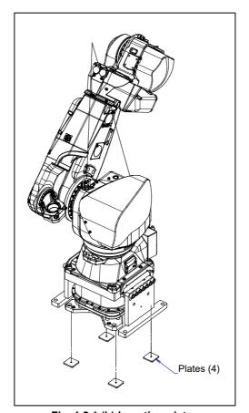
Fig. 1.2.1 (b) Inserting plates
