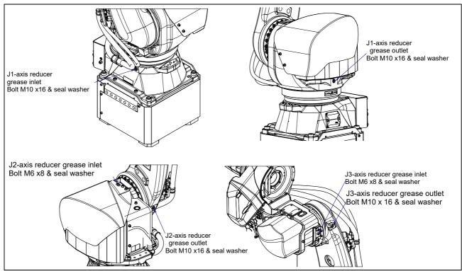
Fig. 7.3.2.1 (a) Greasing point of J1/J2/J3-axis reducer
