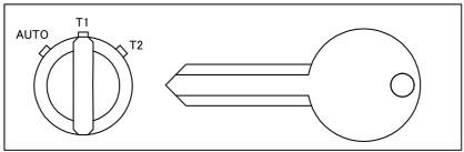
Fig. 4.3 (a) Example of mode select switch
