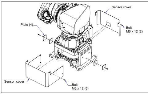
Fig. 1.2.1 (a) Removing the plate and the sensor cover
