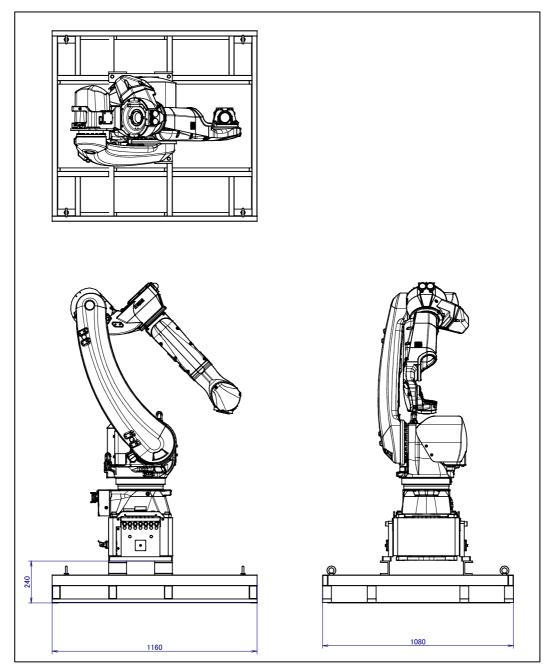
Fig.1.1 (f) Dimensions of the skid
