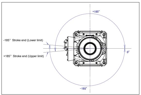
Fig. 3.3 (a) J1-axis motion limit
