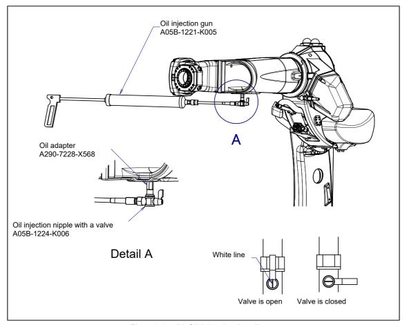
Fig. 7.3.2.4 (b) Oil injection by oil gun
