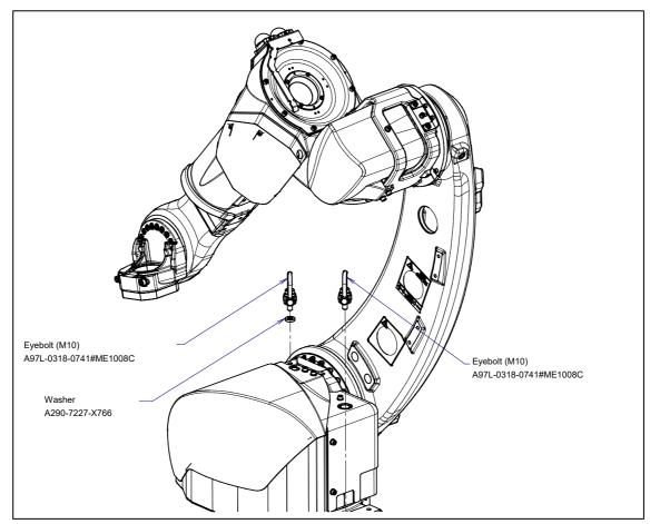
Fig.1.1 (b) Attachment of the transport equipment
