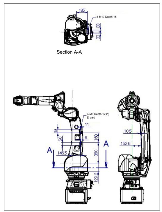
Fig. 4.2 (c) Equipment mounting faces (2/2) (D part + J2 base)
