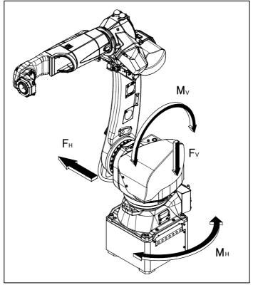
Fig. 1.2.1 (g) Force and moment that acts on the robot base
