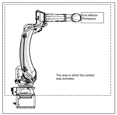
Fig 3.6 (a) Contact stop parts of robot
