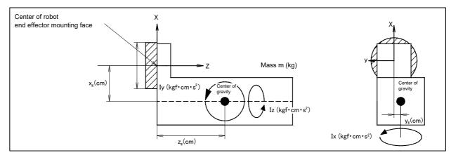
Fig. 4.3 (a) Standard tool coordinate
