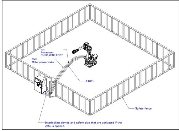
Fig. 2.4.2 (a) Safety fence and safety gate
