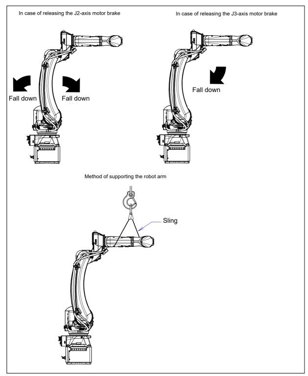
Fig. 5.10 (a) Releasing J2 and J3 motor brake and measures
