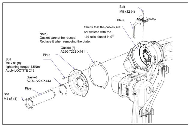
Fig. 8.1 (b) Confirming the state of cable (J4-axis)
