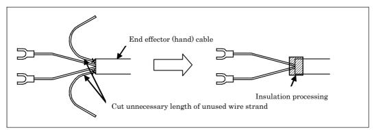
Fig. 5 (a) Treatment method of end effector (hand) cable
