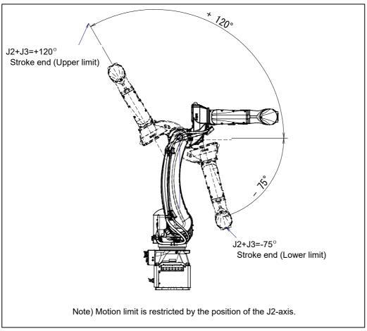
Fig. 3.3 (c) J3-axis motion limit
