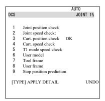
5 Move the cursor to [1 Joint position check], then press the [DETAIL].
