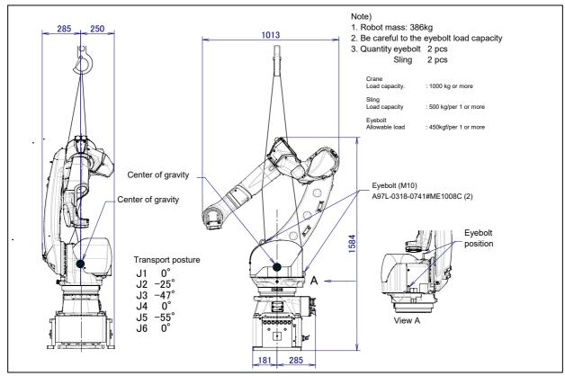
Fig. 1.1 (c) Transportation using a crane
