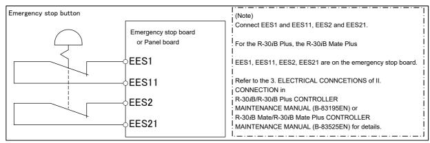
Fig. 2.4.4 (a) Connection diagram for external emergency stop button
