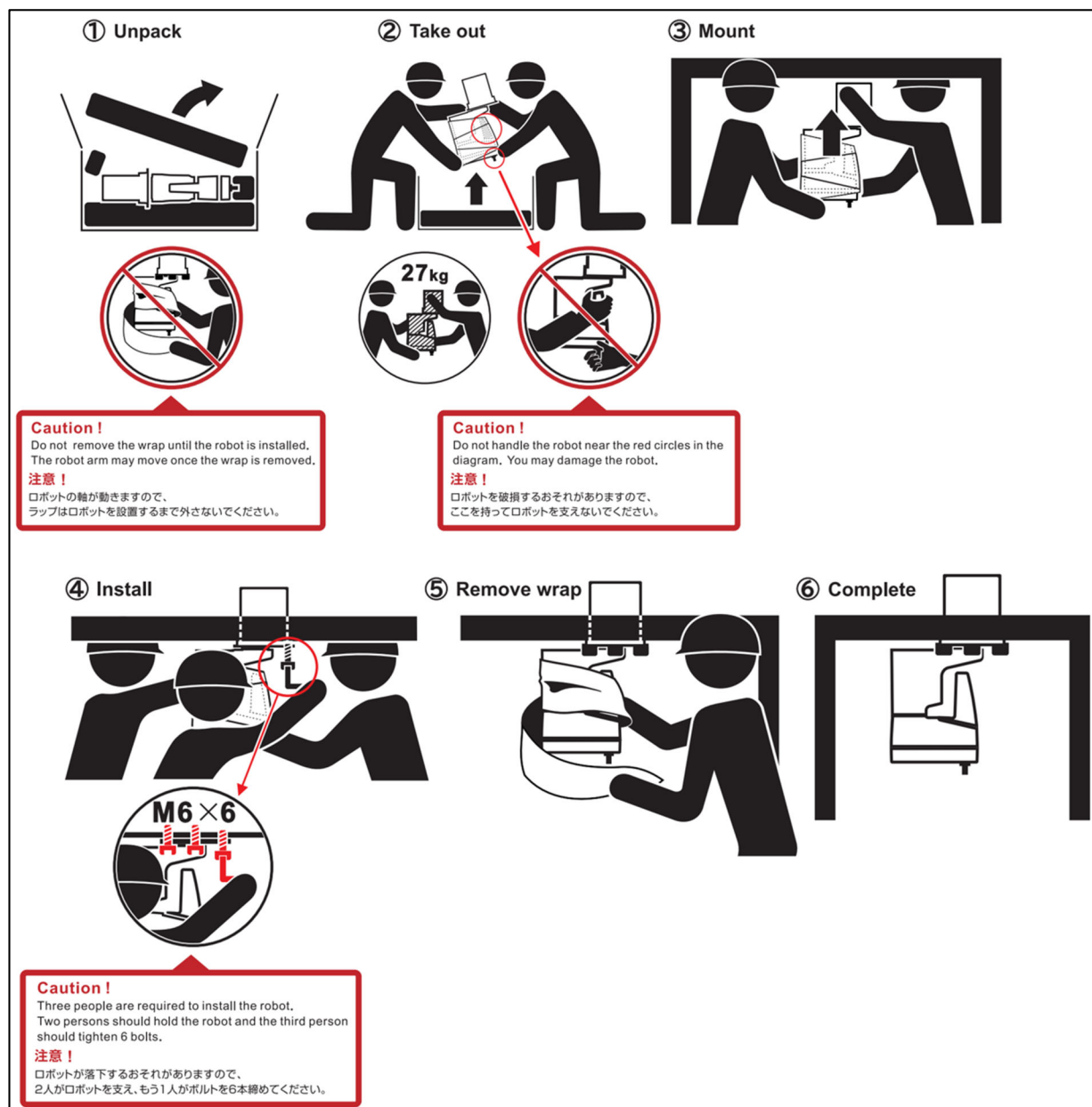
Fig. 1.1 (b) Installing method
