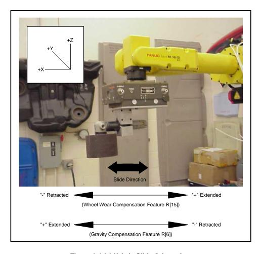
Figure 2.4 (a) X Axis Slide Orientation
