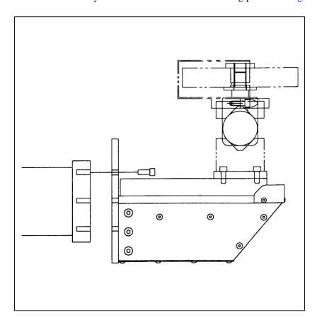
Figure 2.1.2 (a) Active Force Control Device Installation
