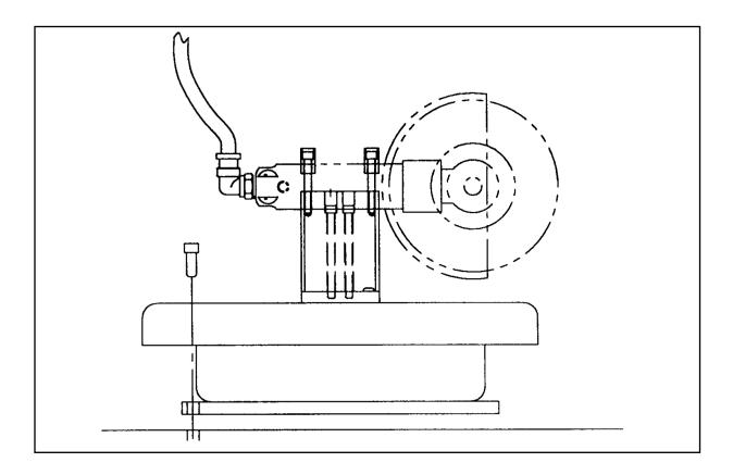
Figure 2.1.2 (c) Passive Bench Mounted Device Installation
