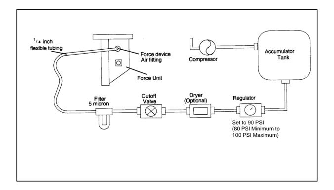
Figure 2.1.3 Active Force Control Device Pneumatic Connections
