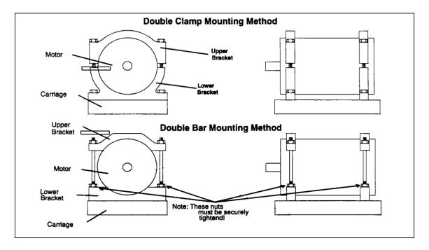
Figure 2.1.1 Double Clamp Mounting Method
