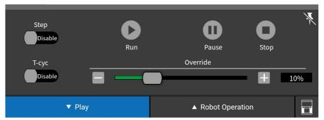
Fig. 3.1.3(b) Displaying Execution Panel
