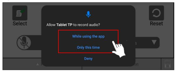
If audio recording is allowed, the Production screen will be display with voice recognition enabled. The Execution panel, the Robot Operation panel, and Key Sheet cannot be displayed on the Production screen. The description and usage of each icon is described in Table 5.2.2.
