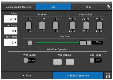
Fig. 9.8.3 The Robot Operation panel for arc welding
