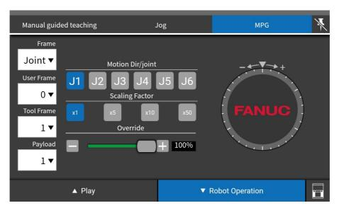
Figure 3.3.2(a) MPG Jog panel(Joint)
