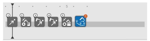
Fig. 9.9.5(h) Arc Handle Teaching with the Multi-pass Weld option
