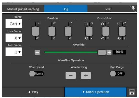
Fig. 9.1(a) The "Robot Operation" panel for arc welding
