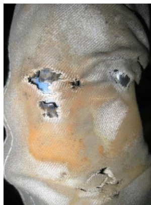
Fig. 7.2.3 (b) Damage on the cable protective sleeve
