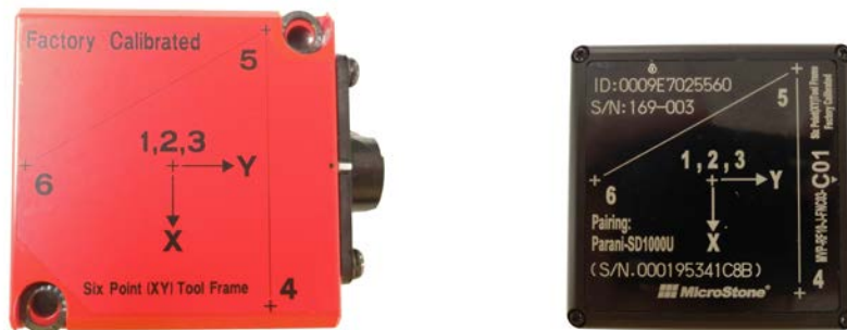
Fig.4(a) Sensor Frame (Left: Wired Accelerometer, Right: Wireless Accelerometer)
