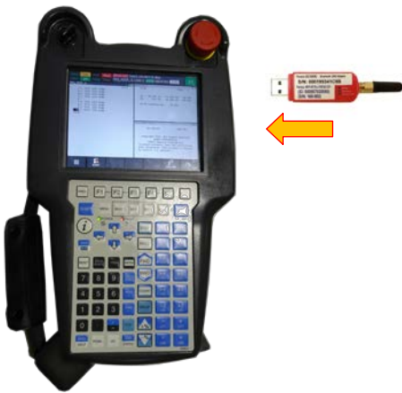
Fig. 2(c) Connection of the USB receiver
