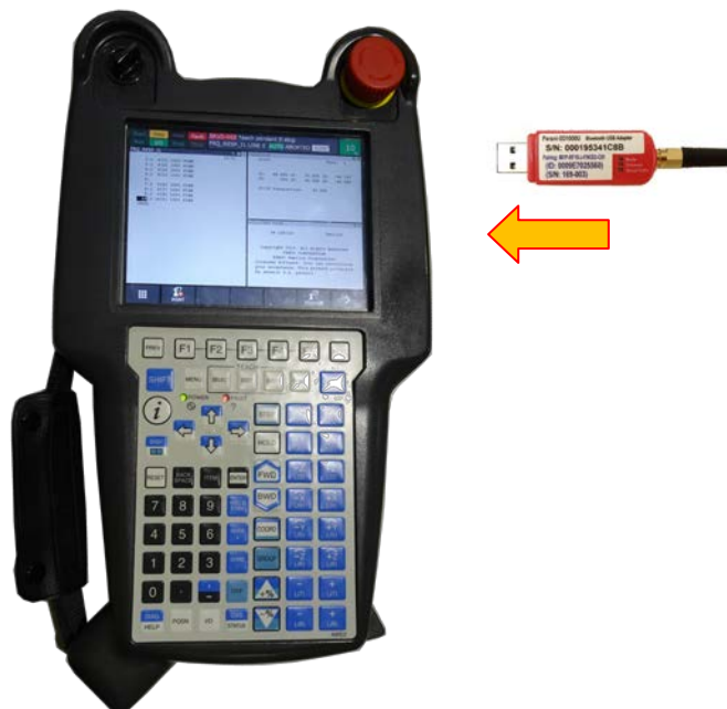
Fig. 3.1.2 (a) Connection of the USB receiver
