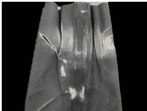
Fig. 7.2.3 (b) Damage on the cable protective sleeve
