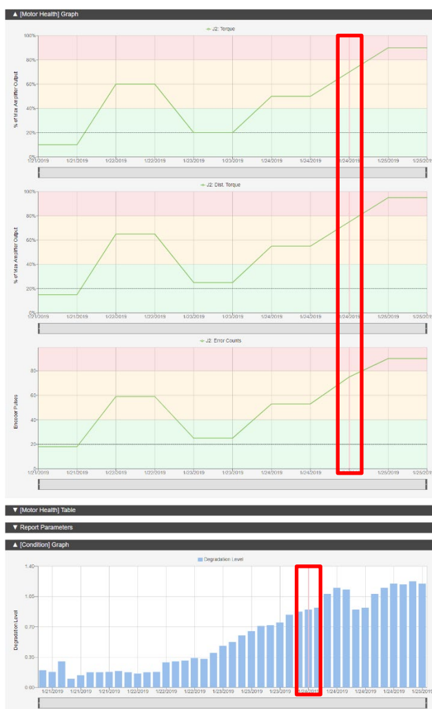
Fig. 3.6.2.2 (d) Red vertical lines display when an error is detected in motor health analysis or PPM-axis analysis
