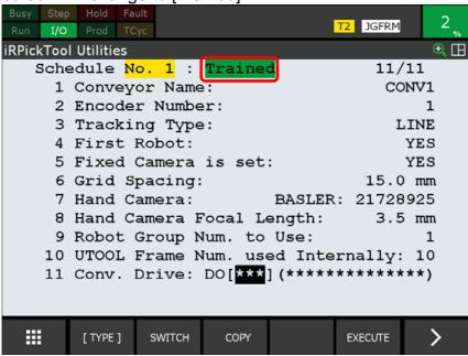
If you are controlling the drive for the conveyor using DO, enter the DO number in [Conv. Drive].
