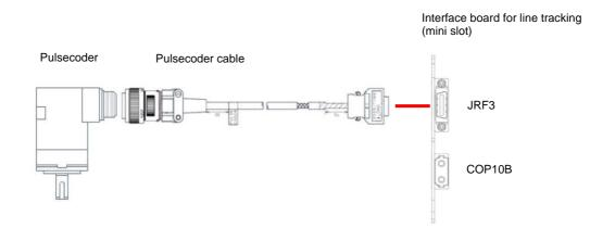
After you have finished connecting, perform setup so that you can control the Pulsecoder from the robot controller.
