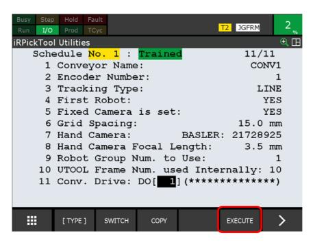
The setup screen for camera calibration will appear.
