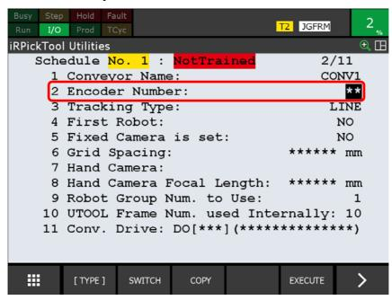
Here, Encoder Number 1, which was set in "2.2 SETTING UP PULSECODER" is entered.
