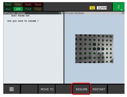
The measurement will be resumed from the location at which it was interrupted.
