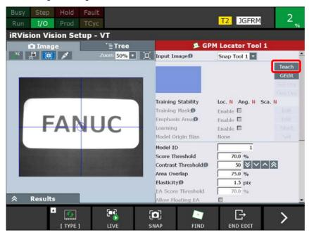
> The screen to teach the model of a workpiece to detect will appear
