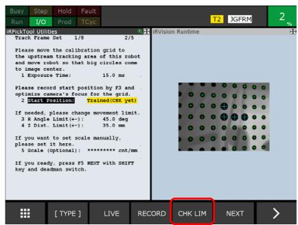
The robot moves by the minimum amount necessary and starts to check whether it can move to the measurement point. When it does this, the robot checks while leaving a margin of about 5 mm in each of the X, Y and Z directions relative to the target position, for safety.
