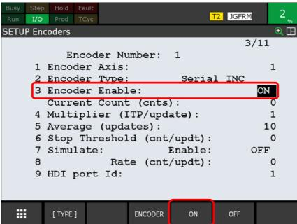
**7.** Move the conveyor and check that the pulse count is updated in [Current Count (cnts)].
