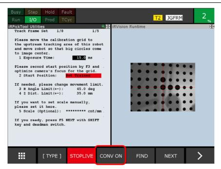
**4.** Move the robot by jog operation so that the large dots are roughly at the center of the image, and adjust the exposure time and focus of the camera.
