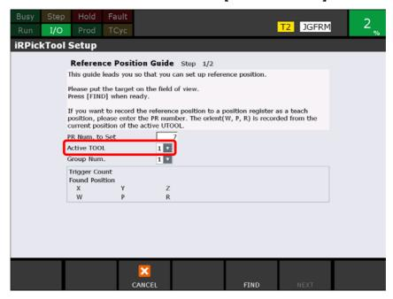
Here, Tool Frame Number 1, which was set in "4 SETTING A TOOL FRAME" is selected.
