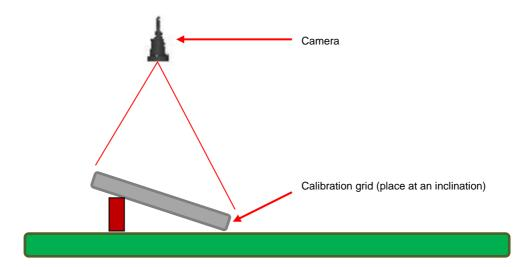
However, for the setup of a tracking frame described later, you must place the calibration grid so it is flat and feed it along. Therefore, press F4 [PREV] on the screen where the detection results are displayed and return to the screen before detection, select [Yes] for [Override Focal Length], place the calibration grid so it is flat, and then proceed to the next step. If you go back to the previous step, the focal length that is retained will be one that has been calculated automatically.
