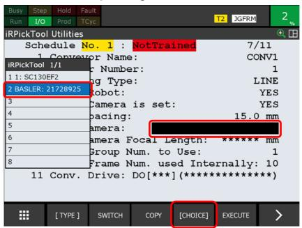
➤ Here, the grid pattern detection camera 'BASLER (USB camera manufactured by Basler (acA640-20um)),' which was mounted on the hand in "1.1.1 Mounting a Grid Pattern Detection Camera," is selected.
