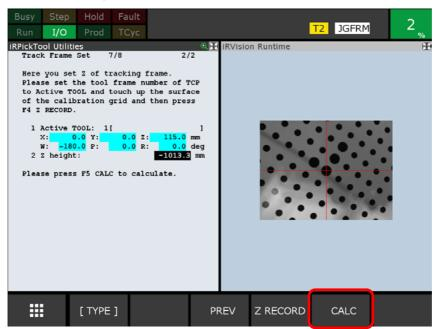
➤ The parameters will be calculated from the measurement results for the first and the second points and [Z height], and the screen will change to a screen for checking the parameter calculation results.
