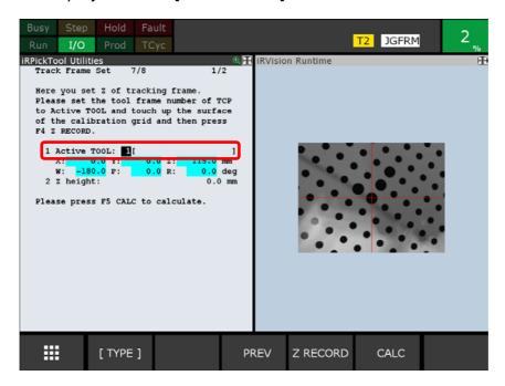
**3.** Move the robot by jog operation, and after it has touched up the surface of the calibration grid, press F4 [Z RECORD].
