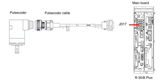
When connecting to the interface board for tracking (mini)
