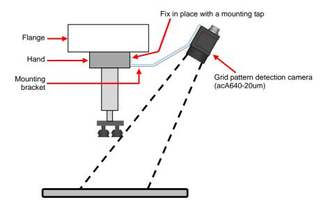
Example 2: Mount the camera using a commercial clamp and flexible arm
