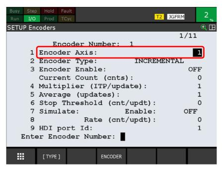
**3.** Move the cursor to [Encoder Type] and press F4 [CHOICE]. From the displayed list, select the encoder type that corresponds to the Pulsecoder that you are connecting.
