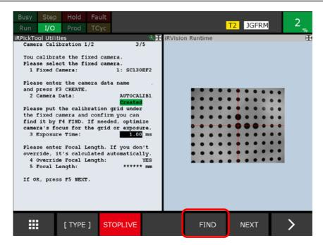
**5.** Move the cursor to [Focal Length], enter the nominal focal length of the lens that you are going to use, and press F5 [NEXT].
