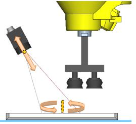
In the direction of the USB camera's field of view, the robot moves up and down by the distance specified in [Z Dist. Limit]. While keeping the dots at the center, the robot rotates by the angle specified in [R Angle Limit].
