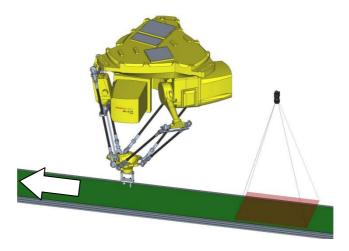
**6.** Place the cursor over [Record] for [Downstream Boundary], and press the [ENTER] key.
