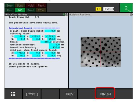
➤ On the basis of the calculation results, robot and conveyor objects will be created automatically, and the [iRPickTool Setup] screen will appear.
