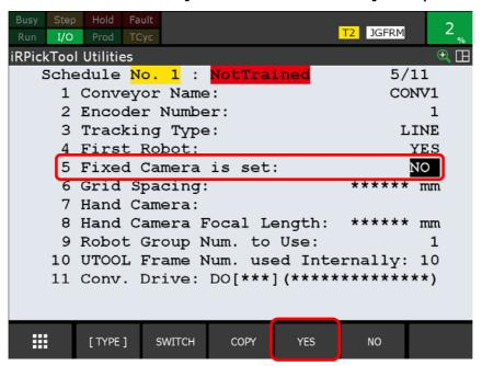
**6.** Move the cursor to [Grid Spacing] and enter the grid spacing.
