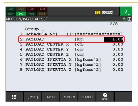
Here, the payload weight is assumed to be 1.0 kg.
