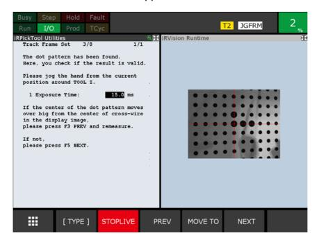
**10.** Rotate the robot around the tool's Z-axis using tool jog operation, and check that the center of the grid pattern is not off the centerline.
