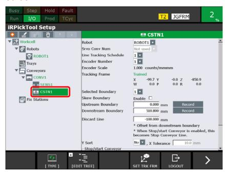
The setup items for the conveyor station will appear on the right side of the screen.
