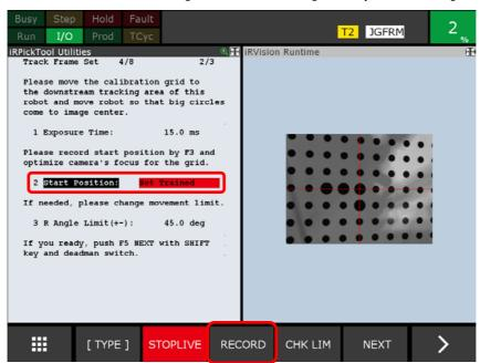
When the position is recorded, the display for [Start Position] changes to [Trained (CHK yet)].
