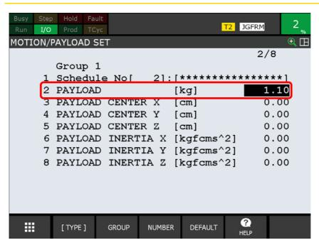
Here, the payload weight is assumed to be 1.1 kg (weight of workpiece: 0.1 kg).
