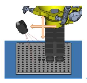
The robot moves all the way in X and Y directions within the range in which the large dots appear in the image.
