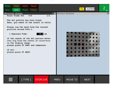
**9.** Rotate the robot around the tool's Z-axis using tool jog operation, and check that the center of the grid pattern is not off the centerline.
