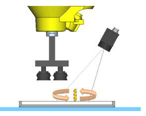
While keeping the dots at the center, the robot rotates by the angle specified in [R Angle Limit].
