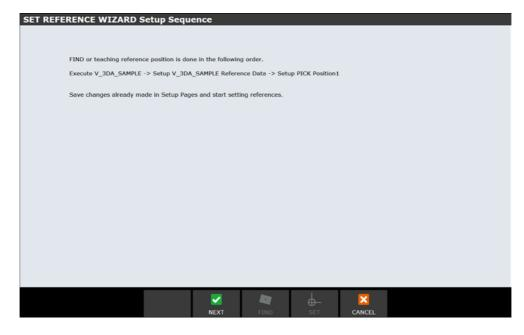
When the following screen for finding a vision process appears, move the robot out of the container by jogging it, for example, place the part at the position where you want to set as the reference position, and click [FIND].
