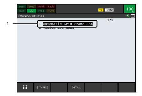
2 Move the cursor to [Automatic Grid Frame Set] and press the [Enter] key. The [Grid Frame Set] page appears.
