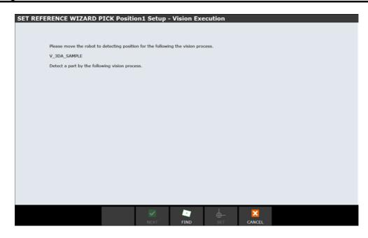
The vision process for SEARCH Vision Process is executed, and the message 'The vision process has run. Please check FIND result in Vision Runtime Page.' shown below is displayed. On the Vision Runtime screen, check that the result of the SEARCH Vision Process is correct, and click [NEXT].
