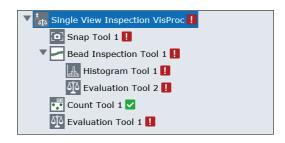
Use 'Bead Inspection Tool 1' to generate inspection points along the sealant. Use 'Histogram Tool 1' to measure the brightness at each inspection point and 'Evaluation Tool 2' to evaluate the result of 'Histogram Tool 1' at each inspection point. Use 'Count Tool 1' to count the number of FAIL and the last 'Evaluation Tool 1' to evaluate the PASS/FAIL for this inspection.
