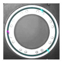
Set [Inspection Interval] you want to inspect in 'Bead Inspection Tool 1'. First, you prepare a work piece with O-ring deviated from the channel, and snap and find in 'Bead Inspection Tool 1'. As a result, you can confirm all of the inspection points plotted on the image. Each cross-hair is an inspection point. Set [Inspection Interval] to create inspection points to detect where the position of the O-ring is misaligned. In this example, [Inspection Interval] is set to 20.
