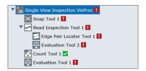
Use 'Bead Inspection Tool 1' to generate inspection points along the sealant. Use 'Edge Pair Locator Tool 1' to measure the width of the sealant on each inspection point and 'Evaluation Tool 2' to evaluate the result of 'Edge Pair Locator Tool 1' at each inspection point. Use 'Count Tool 1' to count the number of FAIL and the last 'Evaluation Tool 1' to evaluate the PASS/FAIL for this inspection.
