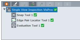
In the example above, the length of the target in the picture taken by 'Snap Tool 1' is measured using 'Edge Pair Locator Tool 1', and the measured length is evaluated using 'Evaluation Tool 1' to evaluate PASS/FAIL.
