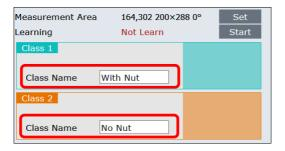
After specifying the class names, set the measurement area for "AI Error Proofing 1" so that the whole welded nut fits into the area.
