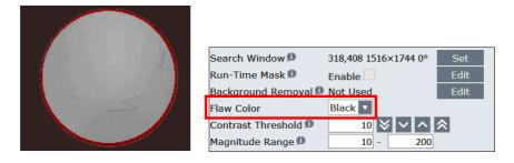
Run a test for multiple button-type batteries using the surface flaw inspection tool to detect the desired scratches.
