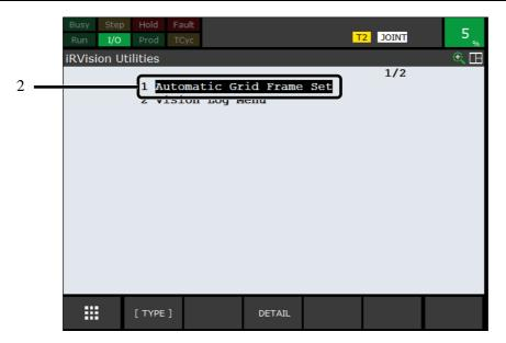
2 Place the cursor over [Automatic Grid Frame Set] and press the [ENTER] key. The [Grid Frame Set] screen will appear.
