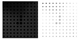
Exposure time too short Exposure time too long Examples of images with inappropriate exposure time
