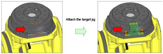
Fig. 7.2.2(c) J6 axis of R-2000*i*B/250F (target fixture)
