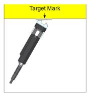
During vision measurement, the relative position of the AMU to the target mark must be kept appropriately by watching the image display. For details, refer to subsection "7.4 IMAGE DISPLAY DURING VISION MEASUREMENT". "Detecting ..." or "Robot is moving ..." is displayed alternately in the bottom of the screen during the measurement.
