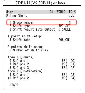
With the 7DF3/11(V9.30P/11) or later software, the robots' group number is set in "Group Number". Select "3PT SFT" (Three point shift) in "Shift Type", then press F1 (START).
