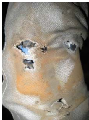
Fig. 7.2.5 (b) Damage on the cable protective sleeve
