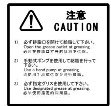
Fig. 4 (a) Greasing and degreasing label
