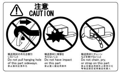
Fig. 4 (m) Transportation prohibitive label (Example of transport equipment option)
