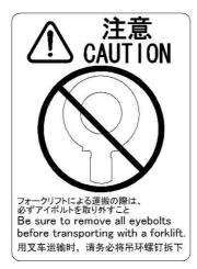
Fig. 4 (o) Transportation caution label (For transport equipment option of R-2000*i*C/165R/210R/100PH/270R J1 base type)
