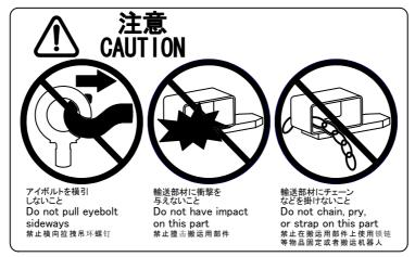
Fig. 4 (I) Transportation prohibitive label (Example of transport equipment option)
