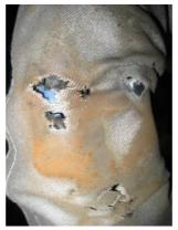
Fig. 7.2.3 (b) Damage on the cable protective sleeve
