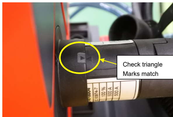
Fig. 7.4 (j) Replacing the torch cable
