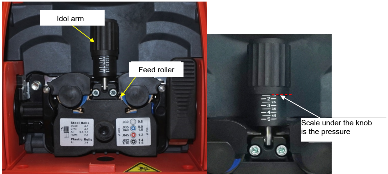
Fig. 5.2.5 (b) Roller pressure adjustment of the wire feeder
