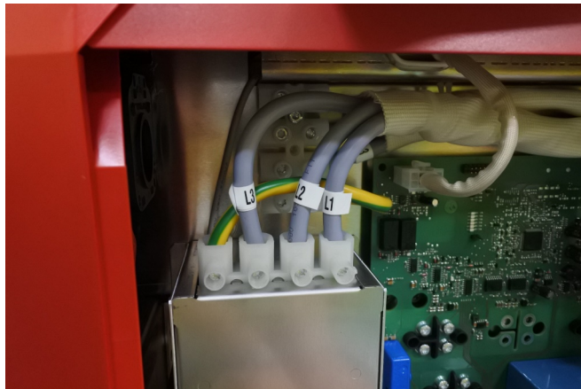
Fig. 2.2.4 (c) Connection of the input power supply
