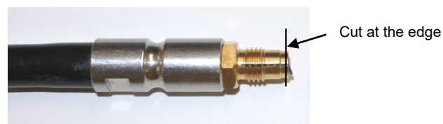
Fig. 5.4.5 (h) Cutting position of the liner
