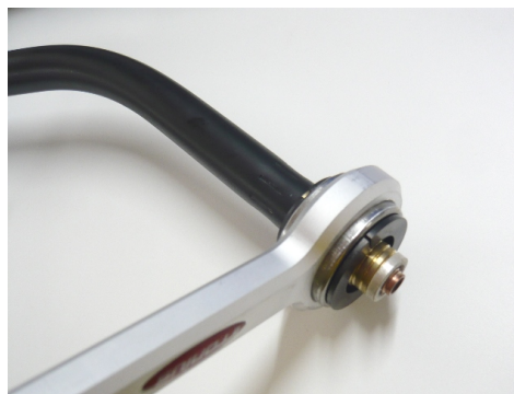
Fig. 7.7 (c) Replacing the nozzle holder
