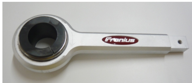
Fig. 7.7 (b) Replacing the nozzle holder
