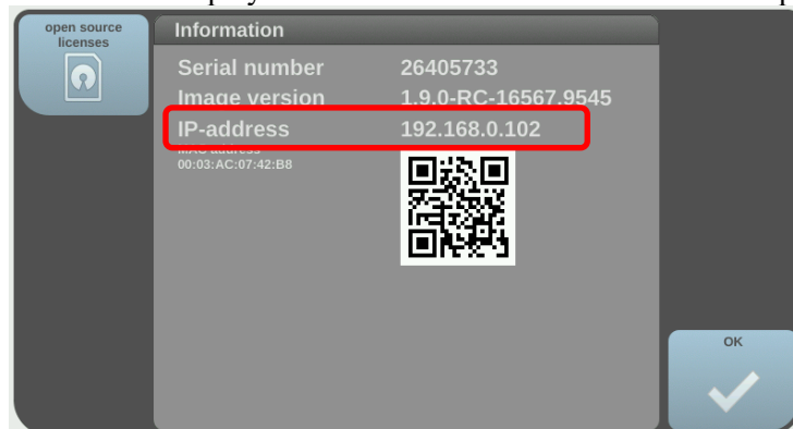
Fig. 6.3.4 (c) IP address of service port
