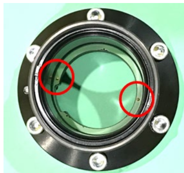
Fig. 6.1.2 (b) Pin inside the crush box
