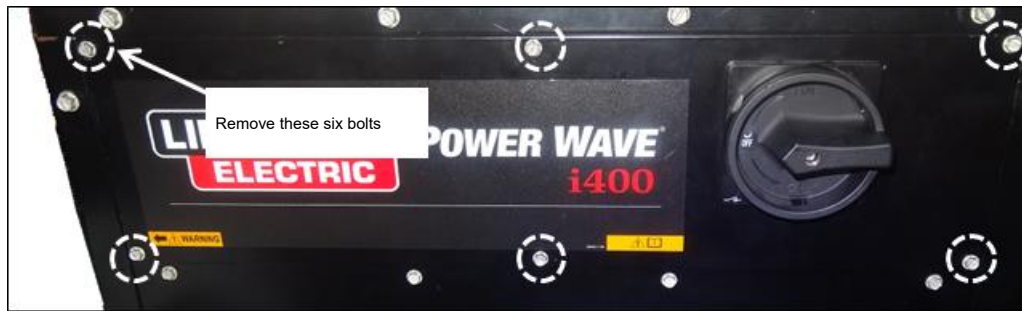
Fig. 7.2 (c) Remove cover of welding power supply
