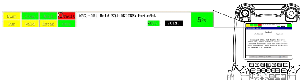
Fig. 2.3 (c) Indication of the connection completion of welding power supply and robot controller
