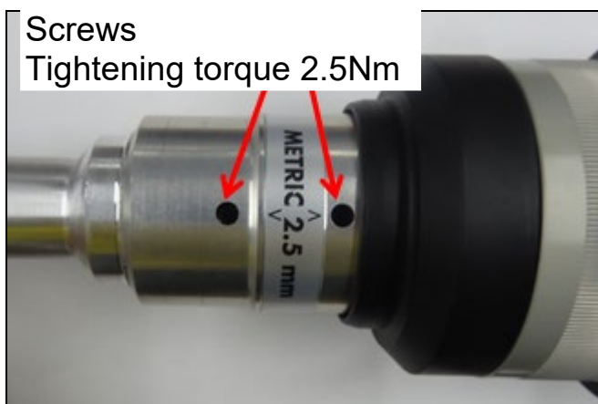
Fig. 7.10 (c) Removing screws
