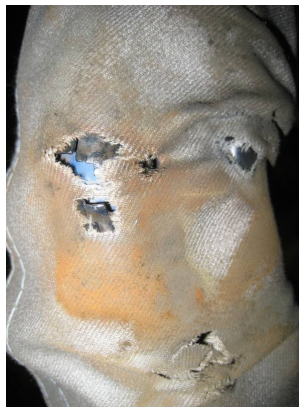
Fig. 7.2.3 (b) Damage on the cable protective sleeve
