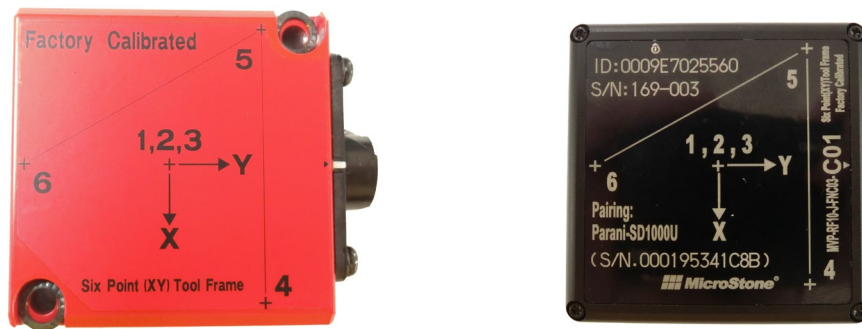
Fig. 3.6(a) Sensor Frame (Left: Wired Accelerometer, Right: Wireless Accelerometer)
