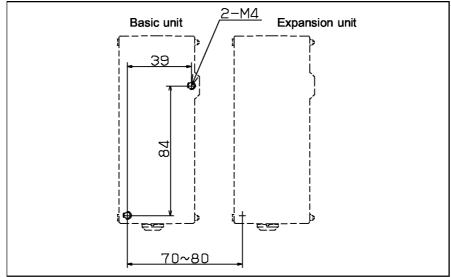
Fig. 2.1.1 (m) Horizontal separation of mounting holes during installation
