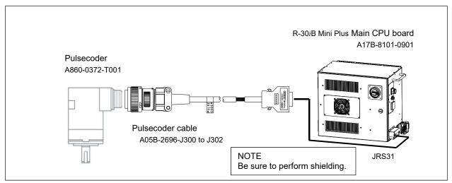
Fig. 2.1.2 (j) Connecting cables with R-30*i*B Mini Plus Main CPU board (one αA1000S Pulsecoder)
