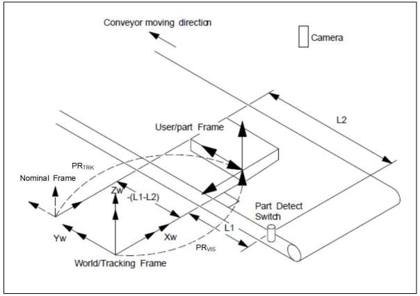
Fig. 5.7.7 User/Part frame and frame relationship in rail tracking system
