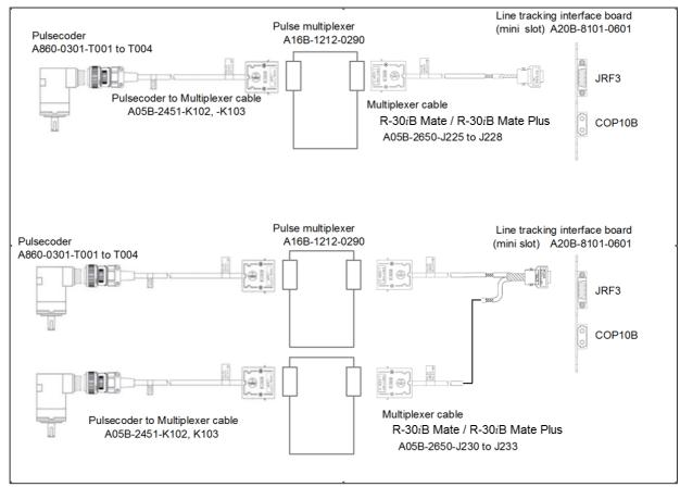
Fig. C.3 (f) Pulse multiplexer and connecting cables 2 (Pulsecoder, A860-0301-T001 to T004)
