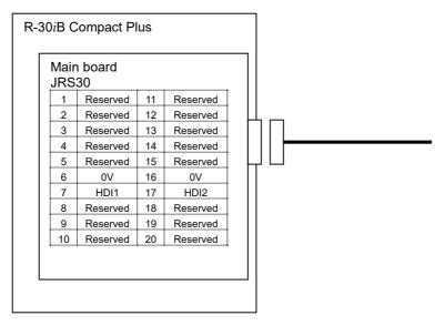
Fig. B.1 (e) R-30iB Compact Plus HDI interface
