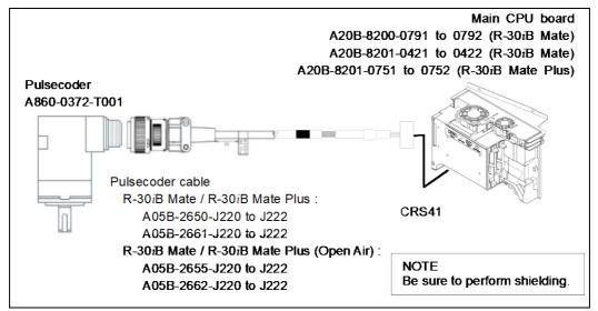
Fig. 2.1.2 (g) Connecting cables with R-30*i*B Mate / R-30*i*B Mate Plus Main CPU board (one αA1000S Pulsecoder)
