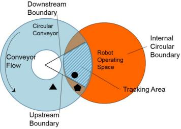
Fig. 5.3(c) Circular Boundary with Circular Conveyor
