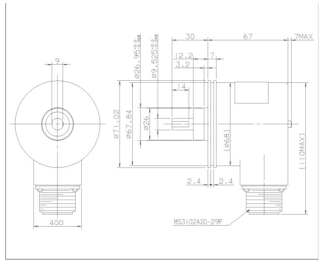
Fig. C.2 (c) Incremental Pulsecoder dimensions (A860-0301-T001)
