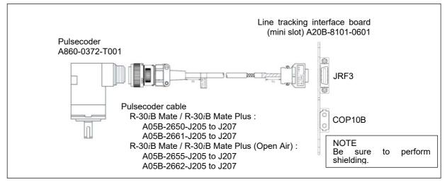
Fig. 2.1.2 (e) Connecting cables with Line tracking interface board A05B-2650-J035, A05B-2655-J035, A05B-2661-J035 or A05B-2662-J035 (one αA1000S Pulsecoder)
