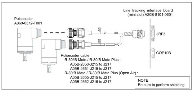
Fig. 2.1.2 (f) Connecting cables with Line tracking interface board A05B-2650-J035, A05B-2655-J035, A05B-2661-J035 or A05B-2662-J035 (two αA1000S Pulsecoders)
