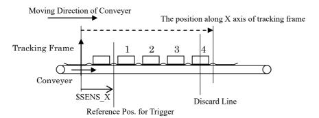
Fig. 6.3.9(h) SLTKDELQ and Stop Conveyor
