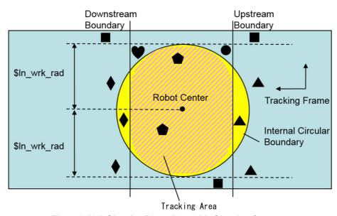
Fig. 5.3.1(a) Circular Boundary with Circular Conveyor
