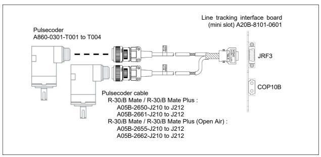
Fig. C.3 (d) Connecting cables with Line tracking interface board A05B-2650-J035, A05B-2655-J035, A05B-2661-J035 or A05B-2662-J035 (two Pulsecoders)
