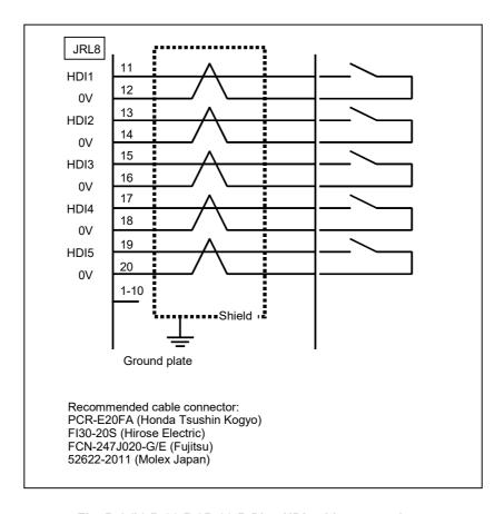
Fig. B.1 (b) R-30iB / R-30iB Plus HDI cable connections
