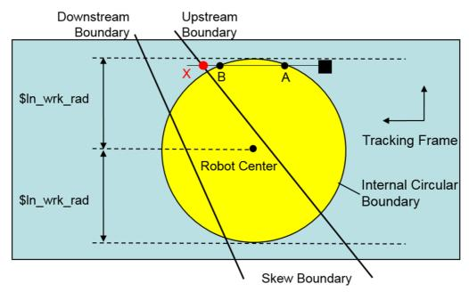
Fig. 5.3.1(b) Part Exits Circular Boundary before Skewed Upstream Boundary
