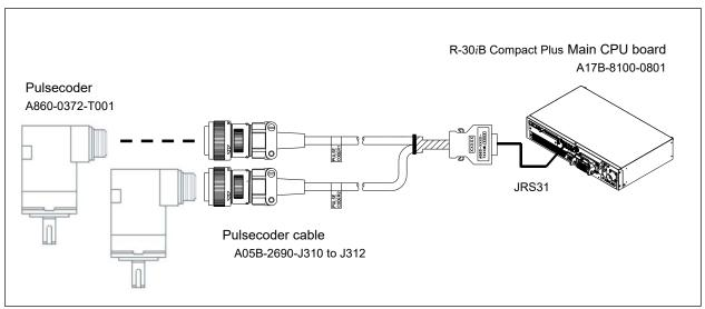
Fig. 2.1.2 (i) Connecting cables with R-30*i*B Compact Plus Main CPU board (two αA1000S Pulsecoder)
