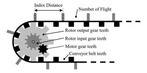
Fig. 6.3.3 Relationship between motor, rotor and conveyor
