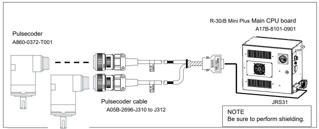
Fig. 2.1.2 (k) Connecting cables with R-30*i*B Mini Plus Main CPU board (two αA1000S Pulsecoder)
