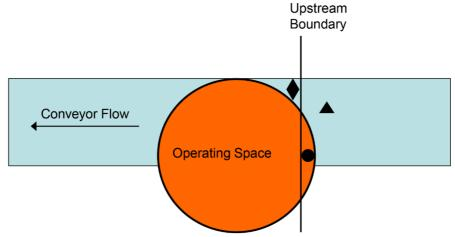
Fig. 5.3(a) Parts Entering the Operating Space of a Robot
