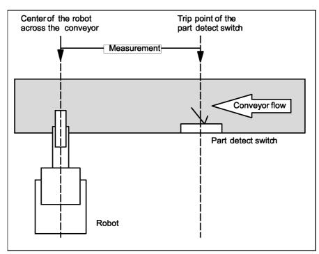
Fig. 3.2(a) Part detect switch (line and rail tracking)
