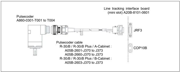
Fig. C.3 (b) Connecting cables with Line tracking interface board A05B-2600-J036, A05B-2660-J036 or A05B-2600-J037 (one Pulsecoder)
