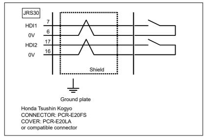
Fig. B.1 (f) R-30iB Compact Plus HDI cable connections
