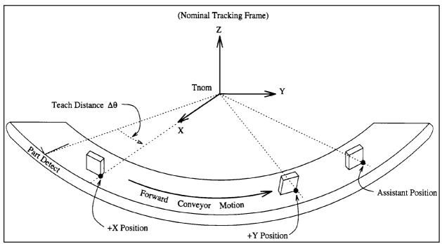
Fig. 3.2.1(b) Nominal tracking frame - counter clockwise circular tracking
