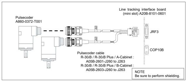
Fig. 2.1.2 (c) Connecting cables with Line tracking interface board A05B-2600-J036, A05B-2660-J036 or A05B-2600-J037 (two αA1000S Pulsecoders)
