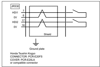
Fig. B.1 (h) R-30iB Mini Plus HDI cable connections
