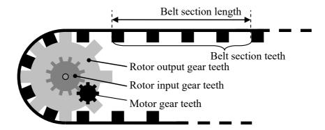
Fig. 6.4.3 Relationship between motor, rotor and conveyor
