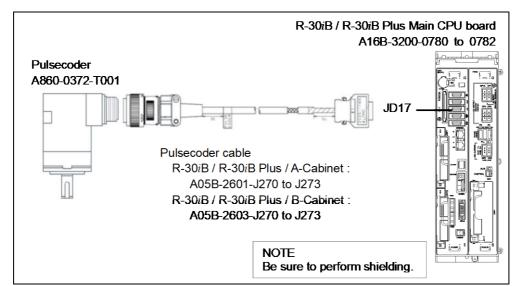
Fig. 2.1.2 (d) Connecting cables with R-30iB / R-30iB Plus Main CPU board (one αA1000S Pulsecoder)
