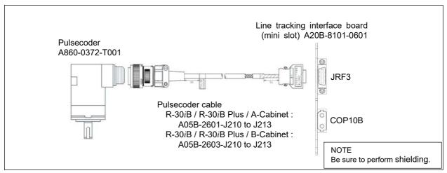
Fig. 2.1.2 (b) Connecting cables with Line tracking interface board A05B-2600-J036, A05B-2660-J036 or A05B-2600-J037 (one αA1000S Pulsecoder)
