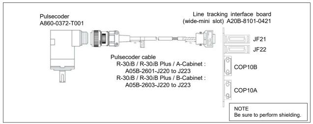
Fig. 2.1.2 (a) Connecting cables with Line tracking interface board A05B-2600-J035 or A05B-2660-J035 (one αA1000S Pulsecoder)
