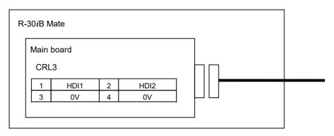
Fig. B.1 (c) R-30iB Mate / R-30iB Mate Plus HDI interface
