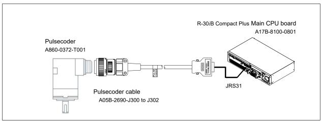
Fig. 2.1.2 (h) Connecting cables with R-30iB Compact Plus Main CPU board (one αA1000S Pulsecoder)
