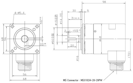
Fig. 2.1.1 (c)  $\alpha$ A1000S Pulsecoder dimensions (A860-0372-T001)
