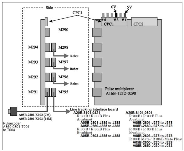
Fig. C.3 (g) Connecting cables to the multiplexer 3 (Pulsecoder, A860-0301-T001 to T004)
