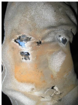
Fig. 7.2.3 (b) Damage on the cable protective sleeve
