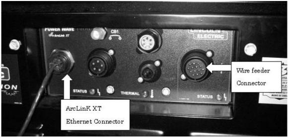
Fig.2.4.1 (b) Connection interface of Welding power supply of ROBOWELD iC/H (Power Wave i400)
