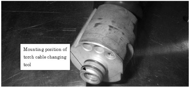
Fig.9.2.1 (h) Mounting position of torch cable changing tool
