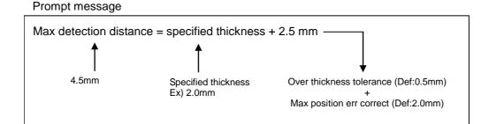
When the above prompt message is displayed, the max detection distance is 4.5 mm. Therefore, the max detection distance is 4.5 mm toward the gun opening direction from the original taught position. If the upper panel is detected at a distance that exceeds the max detection distance, an error (SVGN-240 Up Panel Mis-detect) occurs and the spot program touchup is canceled.
