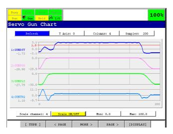
Limit values of disturbance torque during gun closing motion are also displayed.
