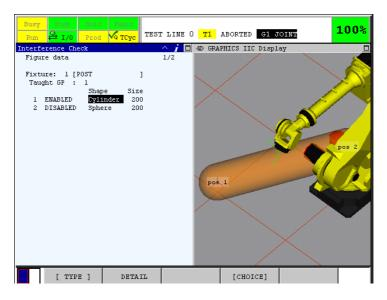
In order to set the cylinder in correct location, press the F2[DETAIL] key and set up X, Y, Z of element 1 of the fixture model.
