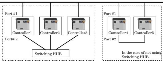
RIPE (Ros Interface Packets over Ethernet) is used for a communication between controllers. It is
