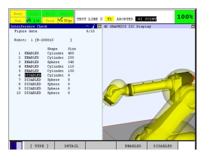
Set up the element data that you would like to add on Element data setup menu. The following is an example that "Cylinder" is added to link 3 of the robot.
