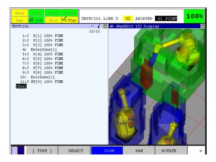
The green spaces are the dead lock zone voxel spaces. To see the relationship between the program and the voxel display, you can turn on the node map on the 4D display by the following step:
