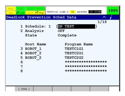
In the Editor menu, press and hold the i key and press the Fctn key at the same time will bring up the relative view menu: Use the Down arrow key to select the 4D IIC Display, the TP becomes
