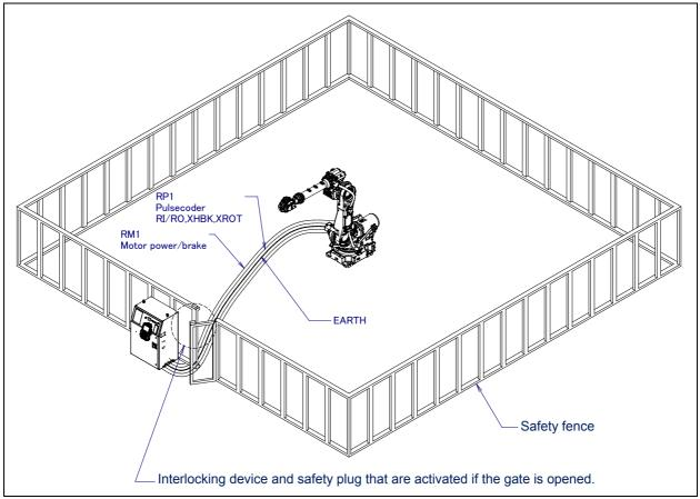
Fig. 3 (a) Safety fence and safety gate
