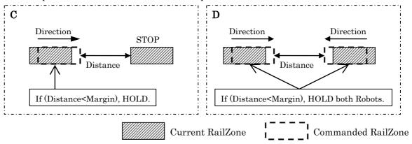
If one robot is moving toward to a rail barrier, the system will hold the moving robot upon detection of the interference between the RailZone and the rail barrier (see E of figure below).
