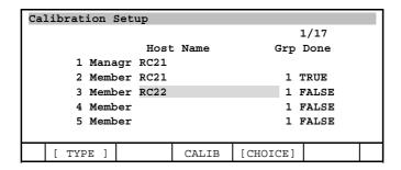
If the origin of group 1 of RC22 is 3000 mm off on the rail, it is necessary to set as the following on Calibration setup. Please set Rail Master Position to 3000 on Rail Robot Setup of RC22 too.
