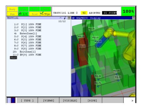
Rotate the 4D graphics and zoom in to the dead lock zones, you can see that by adjusting the taught point points, the robot can avoid the right dead lock zone, and therefore, reduce the possible waiting time.
