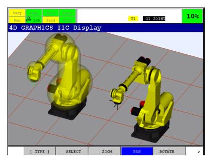
The robot on the left belongs to the first controller that has 4D graphics loaded. The right robot belongs to the second controller that does not have the 4D graphics option.
