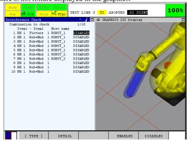
Enable the Fixture 1 on line 1, and the fixture is displayed in the 4D GRAPHICS display.
