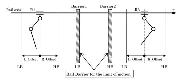
Fig. 3.10.3(b) Example of Rail Barrier
