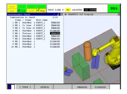
When combination is set to "Critical Zone", a critical zone changes its color from green to red if a robot is inside it. Therefore, you can check where a zone is occupied or not by just looking at the color of the critical zone.
