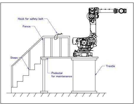
Fig. 3 (c) Pedestal for maintenance
