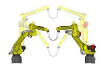
Fig. 3.2.2.2 (a) Example of robots touching TCPs
