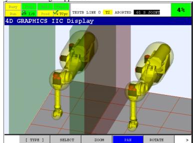
The 2 green planes that surround the left robot is the left and right bound of the left robot. The red plane is the left bound from the right robot. The left and right boundary moves with the left robot, but the right plane does not move unless the right robot moves.
