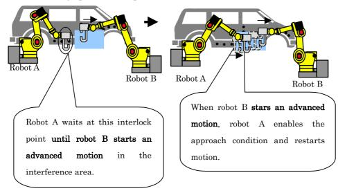
First, ensure by interlocking that robot B moves ahead of robot A. Then, robot A can approaches and waits for robot B.
