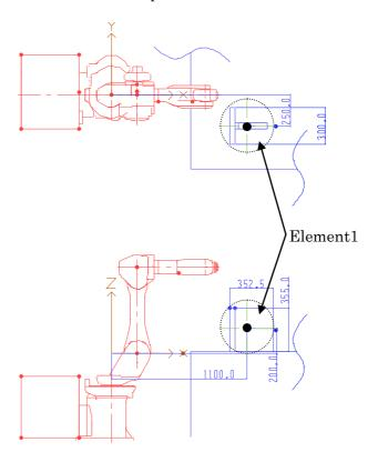
Fig. 3.3.3.1 Sample fixture model
