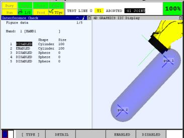
For example, you can change the length of the cylinder to 300mm in Z. The graphics will give you instant visualization feedback of your change after the ENTER key is pressed.
