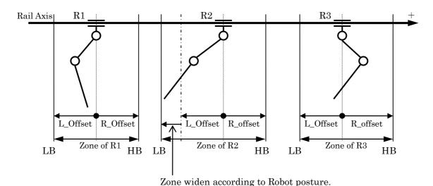
Fig. 3.10.3(a) Example of RailZone
