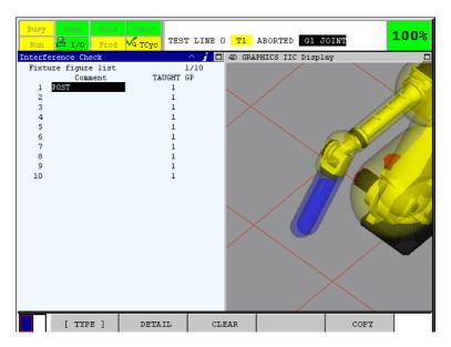
Press F2[DETAIL] key, the fixture model is displayed on the 4D GRAPHICS.
