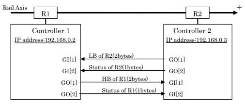
Fig. 3.10.4.5 Example of Communication setup
