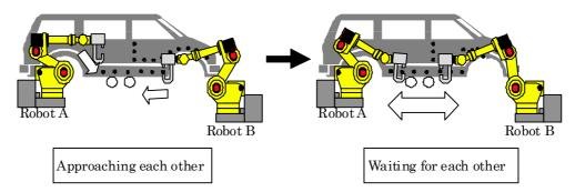
In the example above, robots A and B move to their target points, but the approach waiting function causes both robots to wait.
