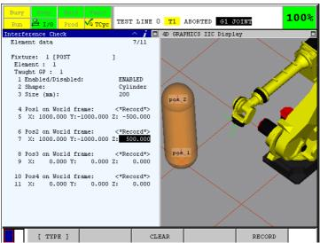
Even if the fixture model is defined, it will not show up in the 4D GRAPHICS display for the whole cell. If the fixture is included in the combination checking, it will show up. Therefore, when leaving the fixture model setup screen, there is not fixture displayed in the graphics.
