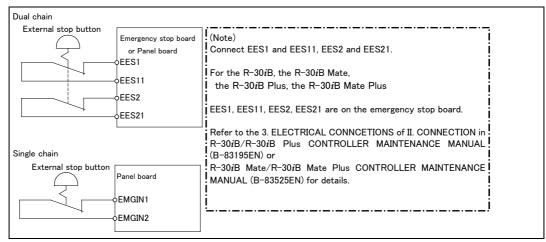
Fig. 3.1 Connection diagram for external emergency stop button
