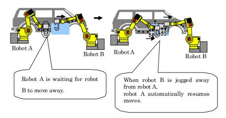
When manually manipulating a robot that moves ahead in a waiting enabled section, ensure that the waiting robot (robot A in the figure above) is held.
