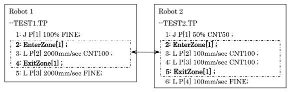
The robot which executes EnterZone[1] first start the next motion instruction. the other robot can not start the next motion instruction and has to wait until ExitZone[1] is executed. When ExitZone[1] is executed, the next motion instruction is started. The same space\_ID (= 1) is specified in both TP programs for relating these instructions.
