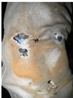
Fig. 7.2.3 (b) Damage on the cable protective sleeve
