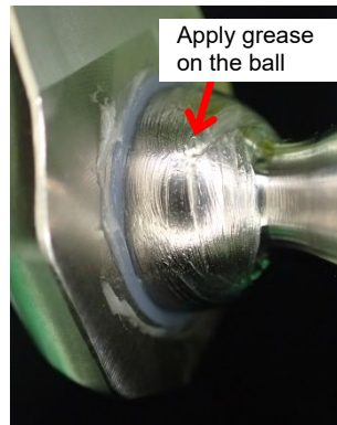
Fig. 6.3.2 (c) Grease applied status
