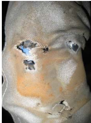
Fig. 7.2.5 (b) Damage on the cable protective sleeve
