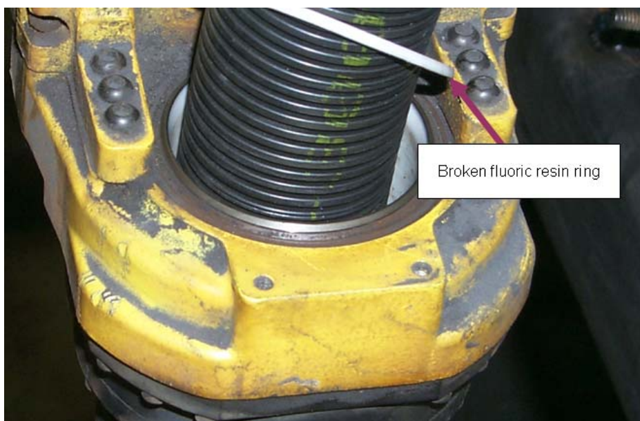
Fig. 7.2.4 (b) Failure of the fluoric resin ring
