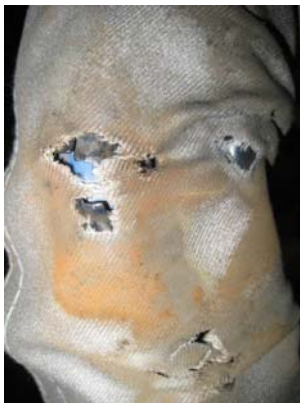
Fig. 8.2.3 (b) Damages on the cable protective sleeve
