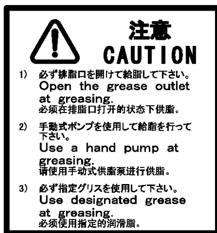
Fig. 4 (a) Greasing and degreasing label
