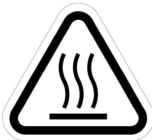
Fig. 4 (e) High-temperature warning label
