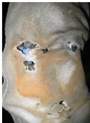
Fig. 7.2.3 (b) Damage on the cable protective sleeve
