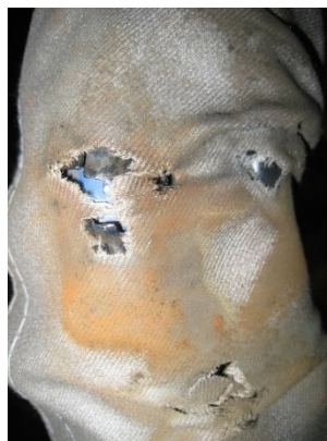
Fig. 7.2.3 (b) Damage on the cable protective sleeve
