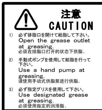
Fig. 7.1 (a) Greasing and degreasing label
