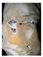
Fig. 8.2.3 (b) Damage on the cable protective sleeve
