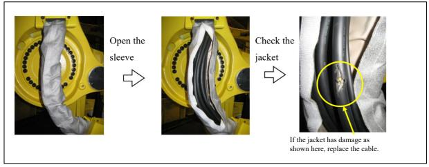
Fig. 7.2.5 (c) Cable check method
