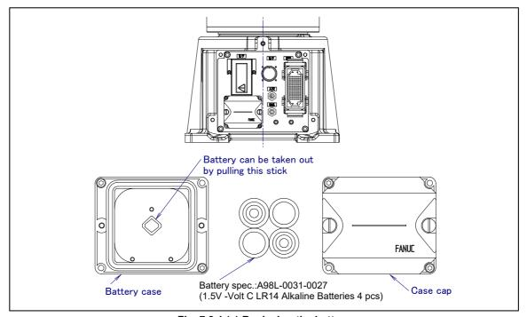
Fig. 7.3.1 (a) Replacing the battery
