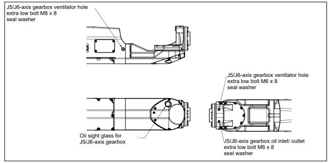
Fig. 7.3.2.4 (b) Greasing point of J5/J6-axis gearbox (ARC Mate 120*i*C, M-20*i*A) (A05B-1225-B251, B252)
