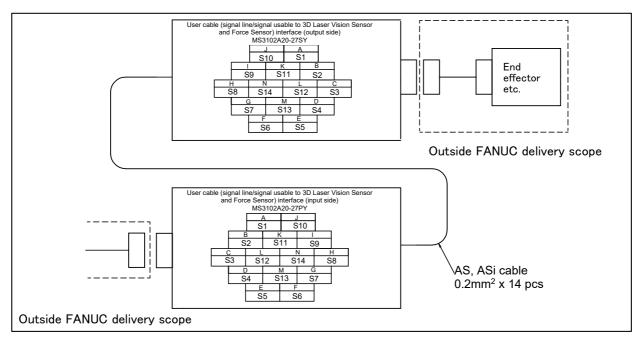
Fig. 5.3 (t) Pin layout for user cable (signal line/signal usable to 3D Laser Vision Sensor and Force Sensor) (AS) (ASi) interface (option)
