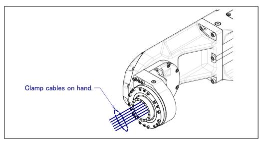
Fig. 11.2 (b) Cabling around wrist
