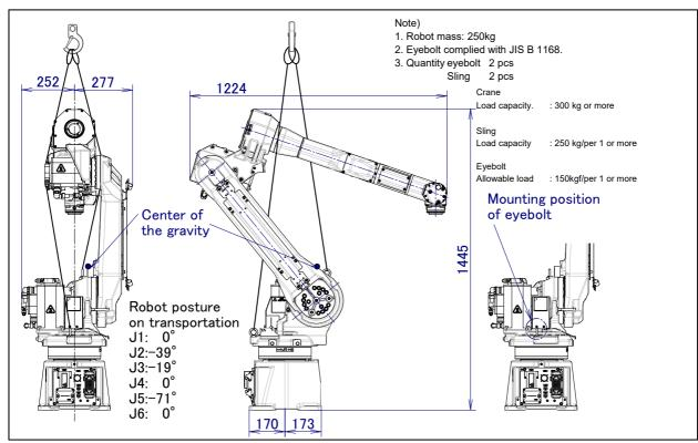
Fig. 1.1 (b) Transportation using a crane (ARC Mate 120iC/10L/12L, M-20iA/10L/12L)
