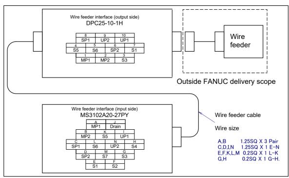
Fig. 5.3 (s) Pin layout for DAIHEN wire feeder (W/F) power supply interface (option)
