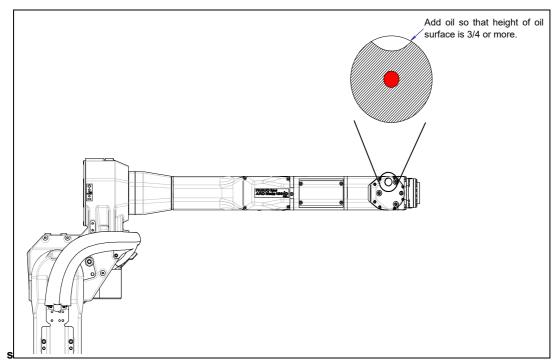
Fig. 7.3.2.5 (e) Standard of oil sight glass (supplying oil for J5/J6-axis gearbox) (ARC Mate 120*i*C/10L, M-20*i*A/10L)
