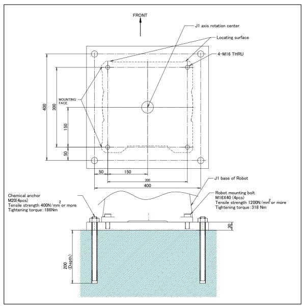
Fig. 1.2.1 (a) Example of installing the robot
