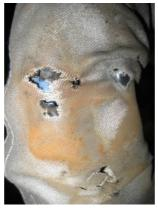
Fig. 7.2.5 (b) Damage on the cable protective sleeve
