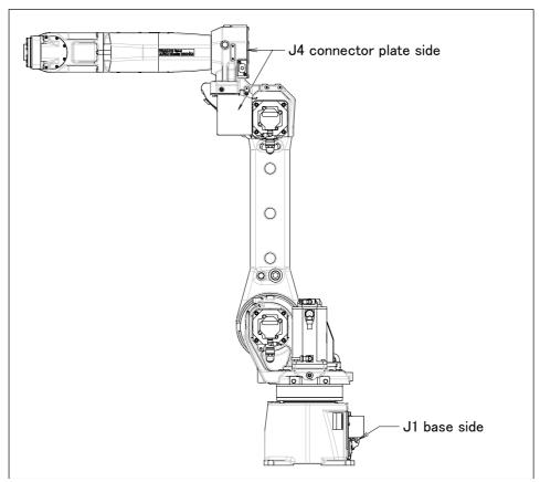
Fig. 5.3 (a) Interface for option cable (Option)
