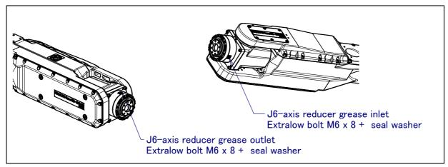
Fig. 8.3.2 (a) J6-axis grease supply position
