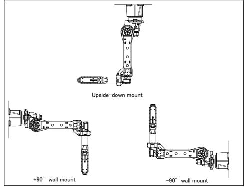
Fig. 8.3.3 (a) Installation method
