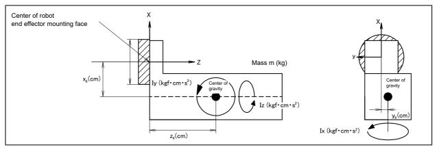
Fig. 4.3 Standard tool coordinate
