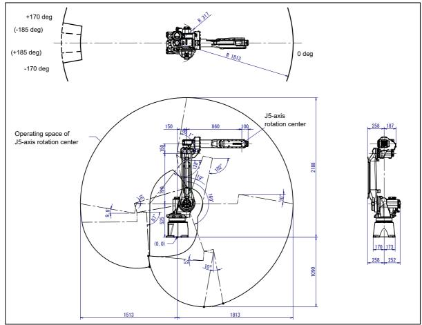
Fig. 3.2 (c) Operating space (M-20*i*A/20M, M-20*i*A/35M)
