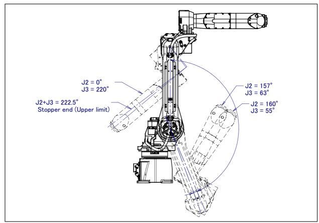
Fig. 3.3 (f) J2/J3-axis motion limit (Upper limit)
