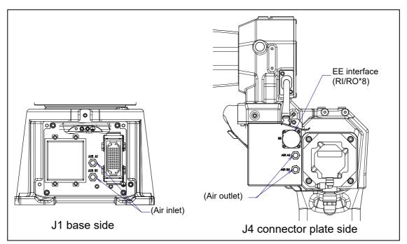
Fig. 5.3 (i) Interface for option cable (A05B-1222-H224 is specified)
