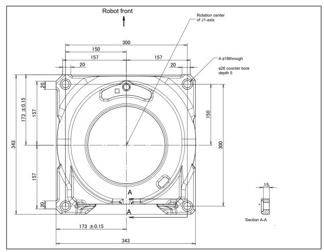
Fig. 1.2 (a) Dimensions of the robot base
