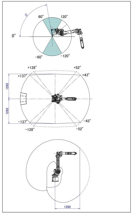
Fig. 3.6 (I) Installation area (3) operating space (M-20*i*A/35M) (-120°<φ<−60°, 60°<φ<120°)
