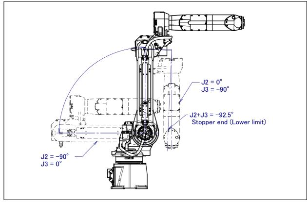
Fig. 3.3 (g) J2/J3-axis motion limit (Lower limit)
