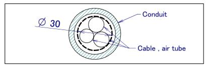
Fig. 12 (b) Outer diameter of cable and air tube in conduit
