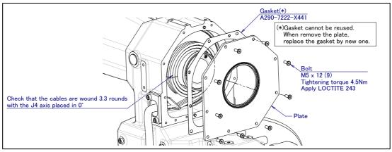
Fig. 9.1 (b) Check the cables statement (J4-axis) (ARC Mate 120iC, ARC Mate 120iC/10L/12L, M-20iA, M-20iA/10L/12L)
