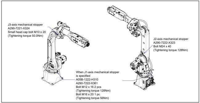
Fig. 8.2.4 (a) Check of mechanical stopper and adjustable mechanical stopper
