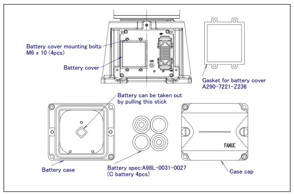
Fig. 7.3.1 (b) Replacing the battery (When severe dust/liquid protection option is specified)
