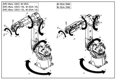
Fig. 3.1 (b) Each axes coordinates and mechanical interface coordinates
