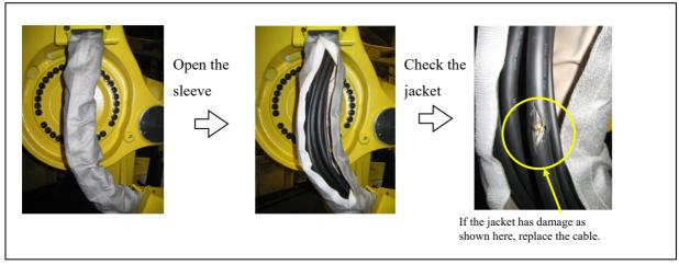
Fig. 8.2.3 (c) Cable check method
