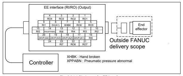
Fig. 5.3 (q) Pin layout for EE interface
