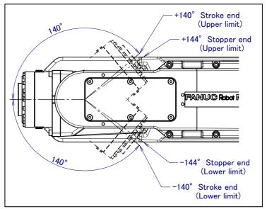
Fig. 3.3 (j) J5-axis motion limit (M-20iA/20M/35M)
