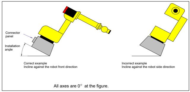
Fig.3.6 (a) Direction of robot wall mount and inclination installation
