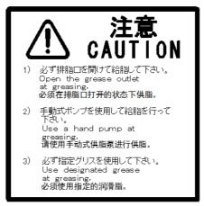
Fig. 4 (a) Greasing and degreasing label
