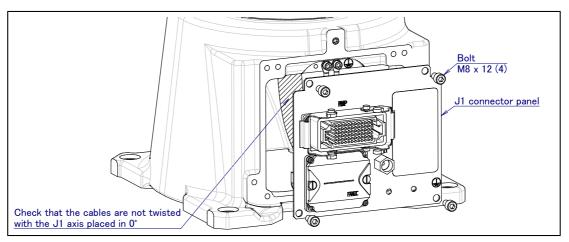
Fig. 9.1 (a) Check the cables statement (J1-axis)
