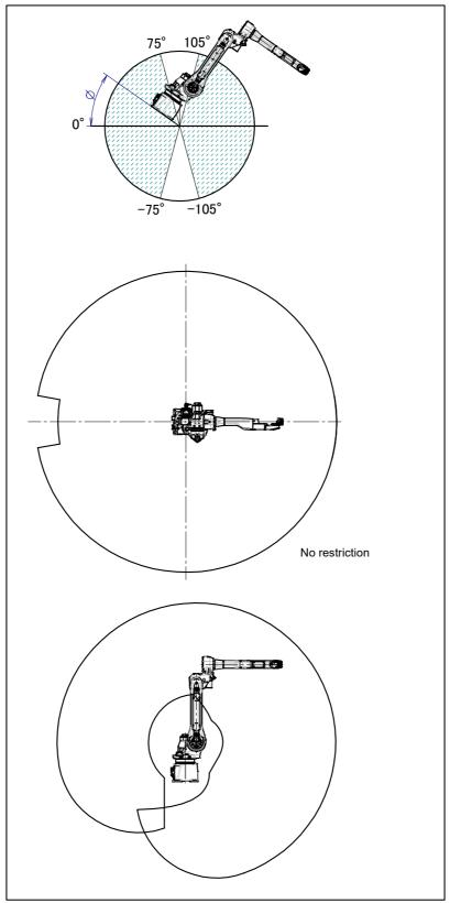
Fig. 3.6 (e) Installation area (1) operating space (ARC Mate 120iC/10L, M-20iA/10L)  $(-180^{\circ} \le \phi \le 105^{\circ}, -75^{\circ} \le \phi \le 75^{\circ}, 105^{\circ} \le \phi \le 180^{\circ})$
