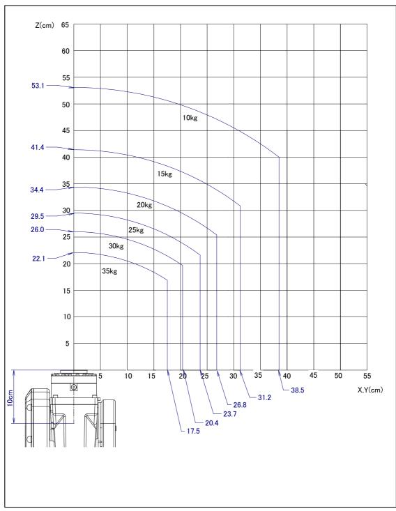
Fig. 3.5 (f) Wrist load diagram (M-20*i*A/35M)
