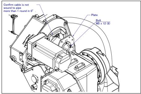
Fig. 9.1 (c) Check the cables statement (J4-axis) (M-20*i*A/20M/35M)
