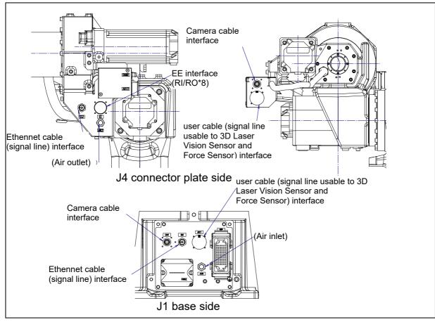
Fig. 5.3 (n) Interface for option cable (A05B-1222-H861 is specified)
