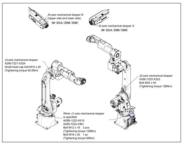
Fig. 3.3 (a) Position of mechanical stopper
