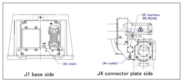
Fig. 5.3 (I) Interface for option cable (A05B-1222-H621 is specified)
