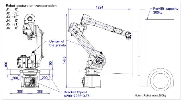
Fig. 1.1 (e) Transportation using a forklift (ARC Mate 120*i*C/10L/12L, M-20*i*A/10L/12L)
