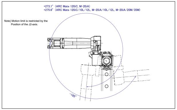
Fig. 3.3 (e) J3-axis motion limit
