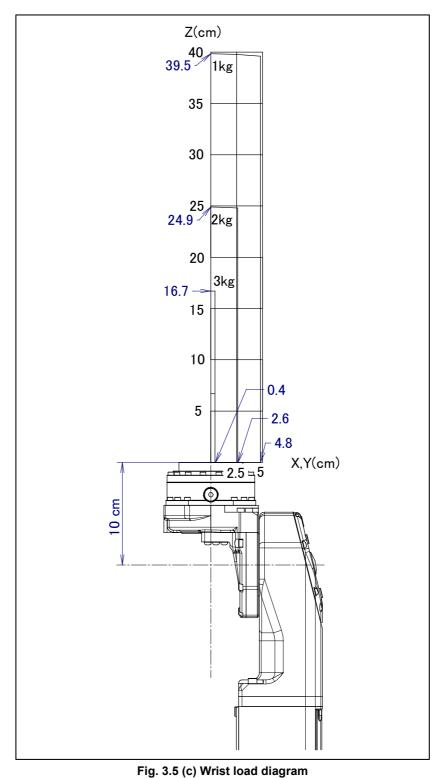
(ARC Mate 120*i*C/10L, M-20*i*A/10L, ARC Mate 120*i*C/12L, M-20*i*A/12L 3kg wrist payload specification)
