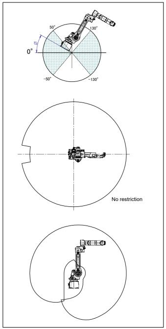
Fig. 3.6 (b) Installation area (1) operating space (ARC Mate 120iC, M-20iA)  $(-180^{\circ} \le \phi \le -130^{\circ}, -50^{\circ} \le \phi \le 50^{\circ}, 130^{\circ} \le \phi \le 180^{\circ})$
