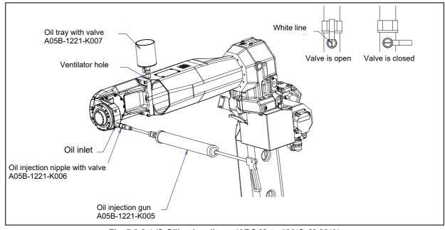
Fig. 7.3.2.4 (f) Oiling by oil gun (ARC Mate 120*i*C, M-20*i*A) (A05B-1225-B251, B252)
