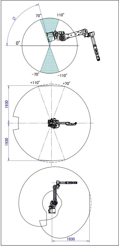
Fig. 3.6 (n) Installation area (2) operating space (ARC Mate 120*i*C/12L, M-20*i*A/12L) (-110°<φ<-70°, 70°<φ<110°)
