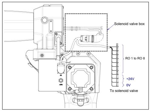
Fig. 11.2 (c) End effector wrist cable relay kit
