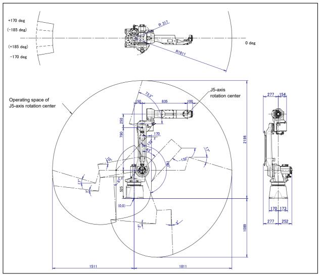
Fig. 3.2 (a) Operating space (ARC Mate 120iC, M-20iA)
