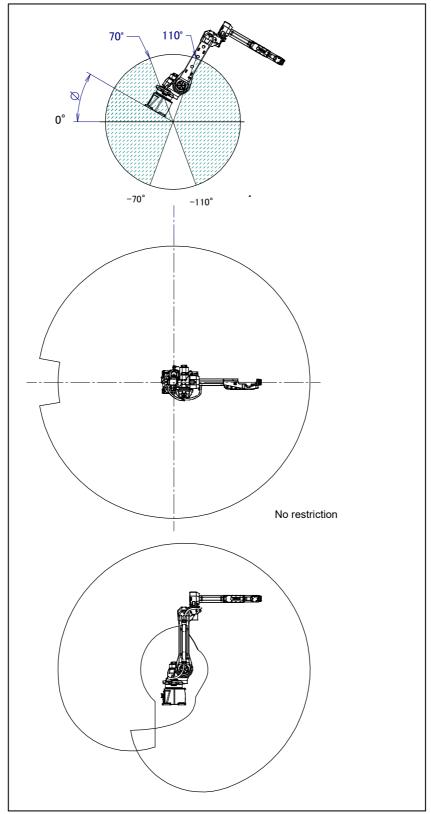
Fig. 3.6 (m) Installation area (1) operating space (ARC Mate 120iC/12L, M-20iA/12L)  $(-180^{\circ} \le \phi \le -110^{\circ} -70^{\circ} \le \phi \le 70^{\circ}$ ,  $110^{\circ} \le \phi \le 180^{\circ}$ )
