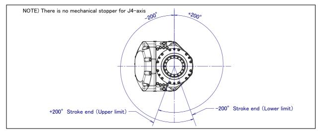
Fig. 3.3 (h) J4-axis motion limit
