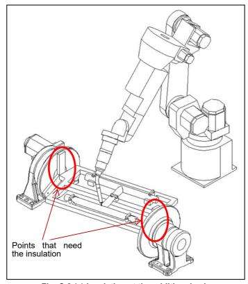
Fig. C.2 (a) Insulation at the additional axis
