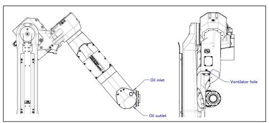
Fig. 7.3.2.4 (c) Oil inlet/outlet and ventilator hole ARC Mate 120*i*C, M-20*i*A) (A05B-1222-B201, B202, A05B-1225-B201, B202)
