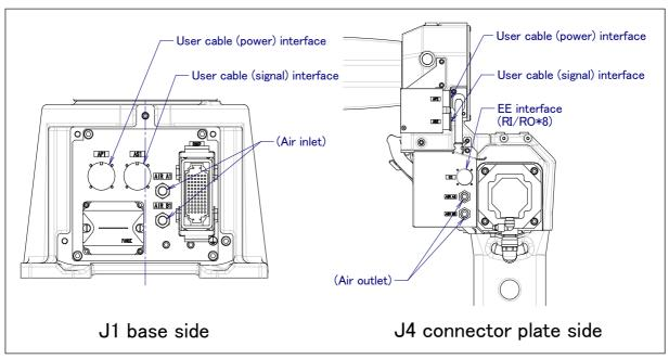
Fig. 5.3 (g) Interface for option cable (A05B-1222-H214 is specified)
