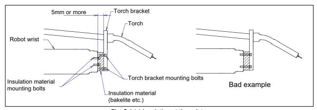
Fig. C.1 (a) Insulation at the wrist
