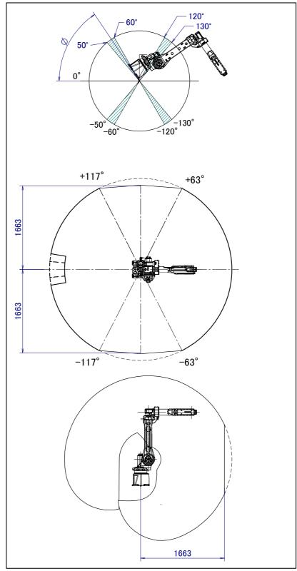
Fig. 3.6 (h) Installation area (2) operating space (M-20iA/20M) (-130°< $\phi$  $\leq$ -120° -60° $\leq$  $\phi$ <-50° 50°< $\phi$  $\leq$ 60°, 120° $\leq$  $\phi$ <130°)
