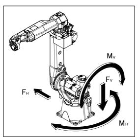
Fig. 1.2.1 (b) Force and moment that acts on the robot base
