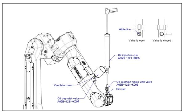
Fig. 7.3.2.4 (e) Oiling by oil gun (ARC Mate 120*i*C, M-20*i*A) (A05B-1222-B201, B202, A05B-1225-B201, B202)
