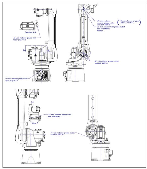
Fig. 7.3.2.1 (a) Greasing point of J1 to J3-axis reducer
