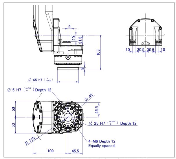
Fig. 4.1 (e) End effector interface (When ISO flange adapter is installed) (ARC Mate 120iC/10L/12L, M-20iA/10L/12L)
