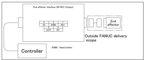
Fig. 5.3 (o) Pin layout for EE interface (RI/RO) RI/RO x 1 (option)
