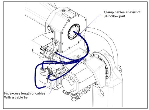
Fig. 11.2 (a) Cabling around J3 casing
