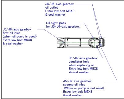
Fig. 7.3.2.5 (a) Oil inlet and outlet (ARC Mate 120iC/10L, M-20iA/10L)
