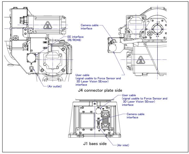
Fig. 5.3 (m) Interface for option cable (A05B-1222-H625 is specified)
