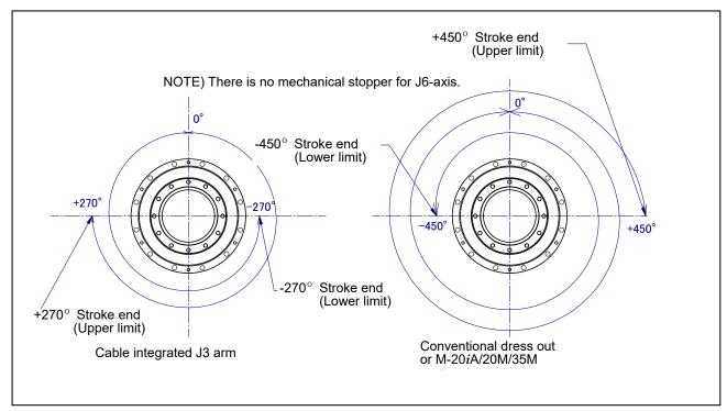
Fig. 3.3 (k) J6-axis motion limit
