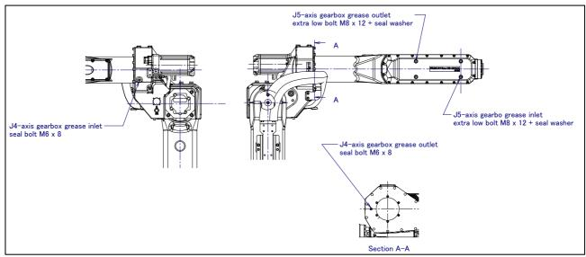
Fig. 8.3.3.2 (a) Greasing point of J4/J5-axis gearbox (M-20*i*A/20M/35M)
