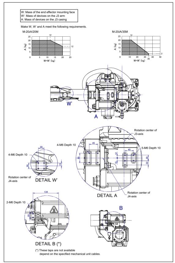
Fig. 4.2 (b) Equipment mounting faces and load limitation (M-20iA/20M/35M)
