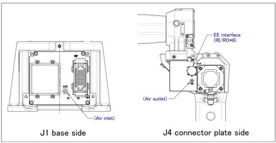
Fig. 5.3 (h) Interface for option cable (A05B-1222-H221, H251, A05B-1225-H251 is specified)
