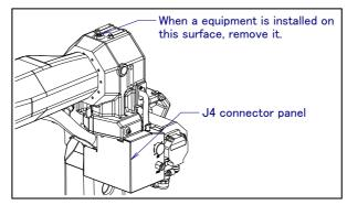
Fig. 7.3.2.3 (b) Removing equipment of the ventilator hole
