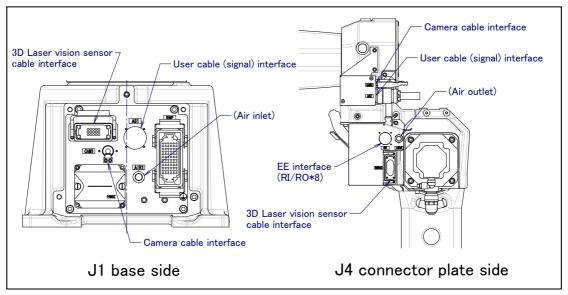
Fig. 5.3 (e) Interface for option cable (A05B-1222-H507, H537 is specified)
