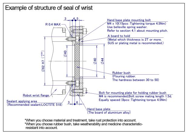
Fig.12 (e) Structure of seal of wrist (example)
