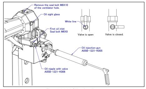
Fig. 7.3.2.3 (c) Oiling by oil gun
