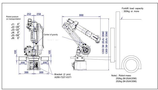
Fig. 1.1 (f) Transportation using a forklift (M-20iA/20M/35M)
