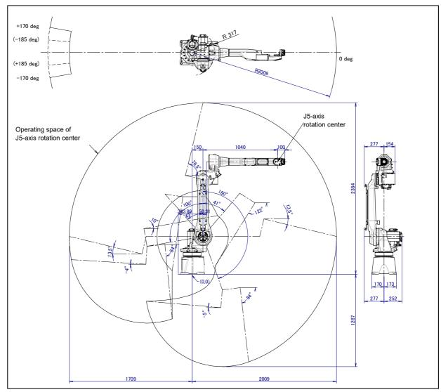
Fig. 3.2 (b) Operating space (ARC Mate 120*i*C/10L, M-20*i*A/10L)
