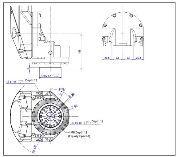
Fig. 4.1 (c) End effector interface (When ISO flange adapter is installed) (ARC Mate 120iC, M-20iA)
