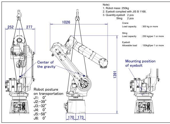
Fig. 1.1 (a) Transportation using a crane (ARC Mate 120iC, M-20iA)
