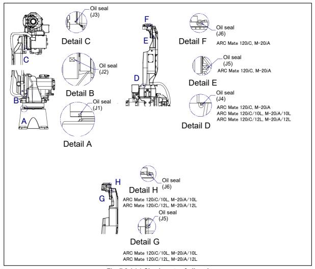
Fig. 7.2.1 (a) Check parts of oil seal
