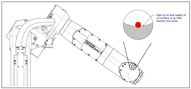
Fig. 7.3.2.4 (g) Standard of oil sight glass (supply oil J5/J6-axis gearbox) (ARC Mate 120iC, M-20iA)
