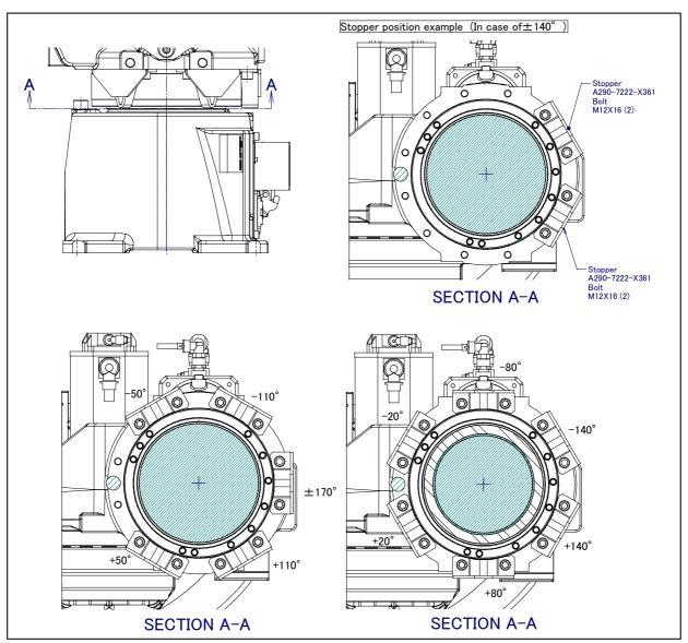
Fig. 6.2 (b) Installing of J1-axis adjustable stopper
