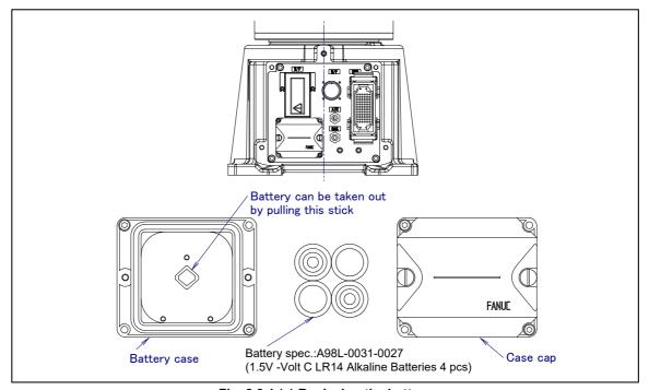
Fig. 8.3.1 (a) Replacing the battery
