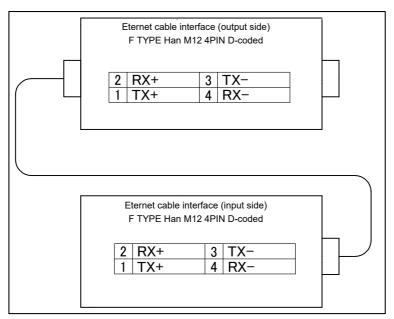
Fig. 5.3 (v) Pin layout for Ethernet (ES) cable interface (option) (When A05B-1222-H861 is specified)
