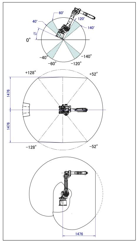
Fig. 3.6 (k) Installation area (2) operating space (M-20*i*A/35M) (-140° $\langle \phi \leq$ -120°, -60° $\leq \phi <$ -40°, 40° $\langle \phi \leq$ 60°, 120° $\leq \phi <$ 140°)
