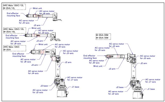
Fig. 3.1 (a) Mechanical unit configuration
