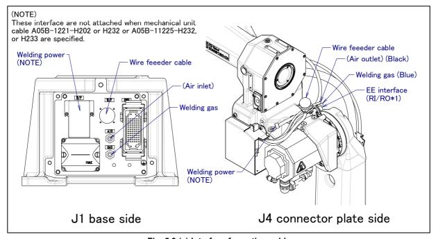
Fig. 5.3 (c) Interface for option cable (A05B-1222-H202, H203, H206, H232, H233, H236, H512, H513, A05B-1225-H232, H233, H236, H532, H533 are specified)
