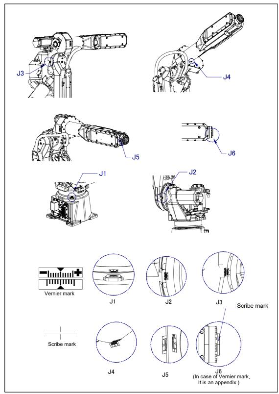
Fig. 9.3 (b) Marking position of each axis (M-20iA/20M/35M)
