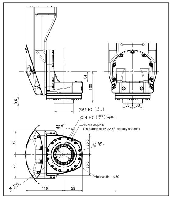
Fig. 4.1 (b) End effector interface (ARC Mate 120*i*C, M-20*i*A) (A05B-1225-B251, B252)
