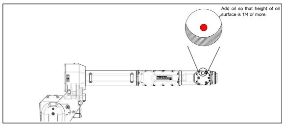
Fig. 7.3.2.5 (f) Standard of oil sight glass (supplying oil for J5/J6-axis gearbox) (ARC Mate 120*i*C/12L, M-20*i*A/12L)
