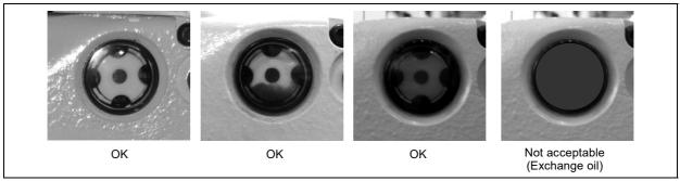
Fig. 7.2.3 (a) The extent of oil deterioration
