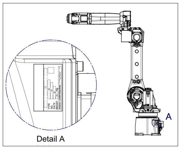
Position of label indicating mechanical unit specification number
