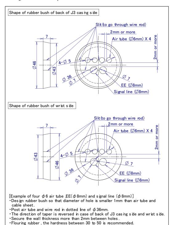
Fig.12 (c) Shape of rubber bush (example)
