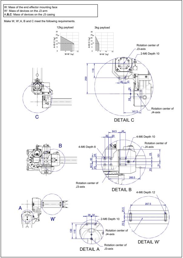
Fig. 4.2 (c) Equipment mounting faces and load limitation (ARC Mate 120*i*C/12L, M-20*i*A/12L)
