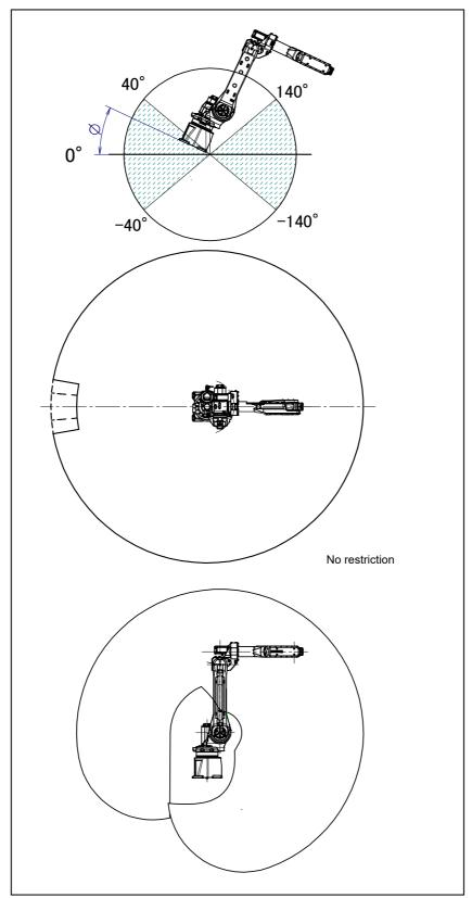
Fig. 3.6 (j) Installation area (1) operating space (M-20iA/35M) (-180° $\leq \phi \leq$ -140°, -40° $\leq \phi \leq$ 40°, 140° $\leq \phi \leq$ 180°)
