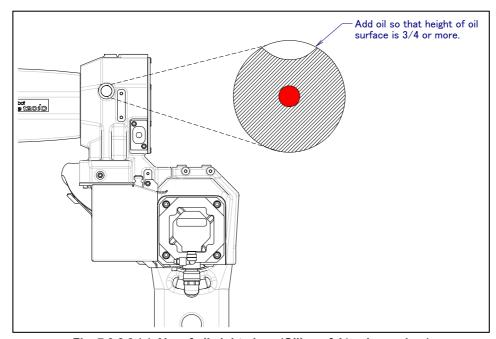
Fig. 7.3.2.3 (e) Aim of oil sight glass (Oiling of J4-axis gearbox)
