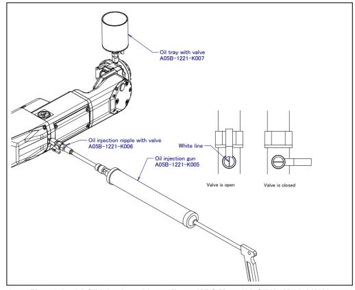
Fig. 7.3.2.5 (c) Oil injection with an oil gun (ARC Mate 120iC/10L, M-20iA/10L)
