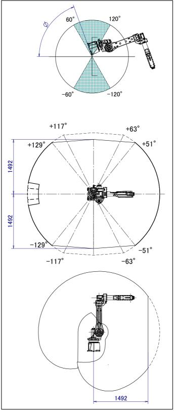
Fig. 3.6 (i) Installation area (3) operating space (M-20*i*A/20M) (-120°<φ<-60°, 60°<φ<120°)
