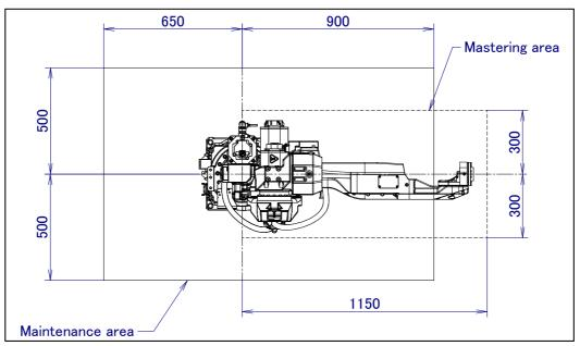
Fig. 1.3 (a) Maintenance area (ARC Mate 120iC, M-20iA)
