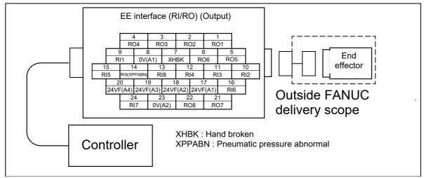
Fig. 5.3 (p) Pin layout for EE interface (RI/RO) RI/RO x 8 (option)
