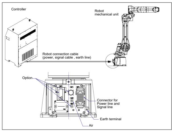
Fig. 2 (a) Cable connection
