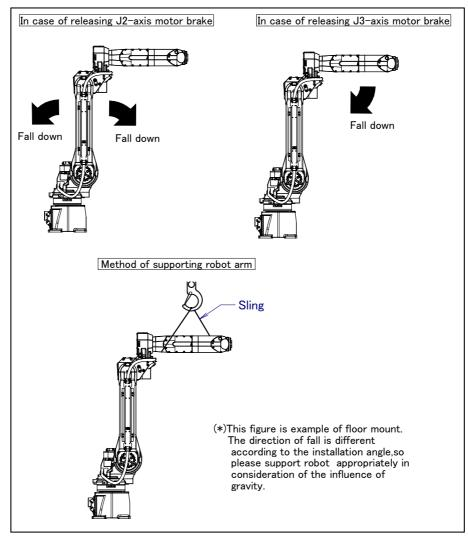
Fig. 3 (a) Arm operation by the release of J2/J3-axis motor brake and measures
