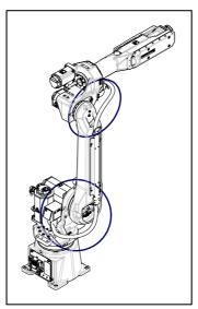
Fig. 8.2.3 (a) Inspection points of the mechanical unit cables
