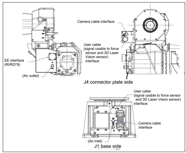
Fig. 5.3 (f) Interface for option cable (A05B-1222-H525, A05B-1225-H255 are specified)
