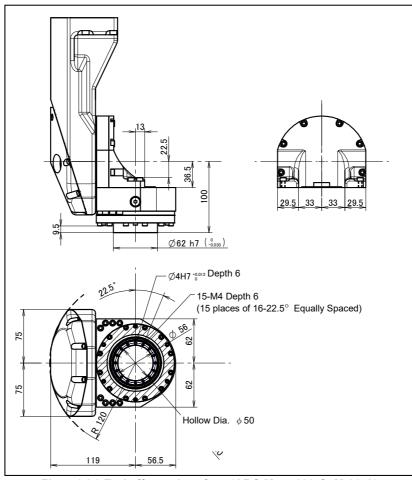
Fig. 4.1 (a) End effector interface (ARC Mate 120*i*C, M-20*i*A) (A05B-1222-B201, B202, A05B-1225-B201, B202)
