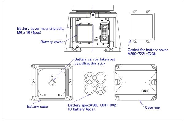
Fig. 8.3.1 (b) Replacing the battery (When severe dust/liquid protection option is specified)
