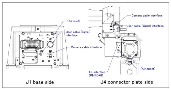
Fig. 5.3 (d) Interface for option cable (A05B-1222-H505, H535, A05B-1225-H235 are specified)
