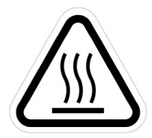
Fig. 4 (c) High-temperature warning label
