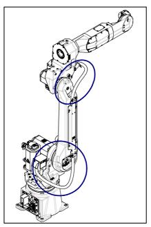
Fig. 7.2.5 (a) Inspection points of the mechanical unit cables
