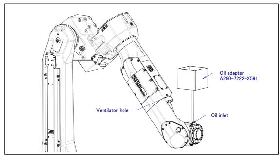
Fig. 7.3.2.4 (h) Oil adapter (for J5/J6-axis gearbox oil inlet) (ARC Mate 120*i*C, M-20*i*A) (A05B-1222-B201, B202, A5B-1225-B201, B202)
