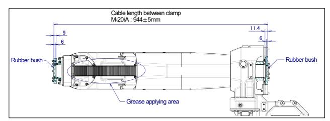
Fig.12 (a) Cable length between clamps
