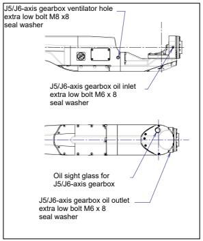
Fig. 7.3.2.4 (a) Greasing point of J5/J6-axis gearbox (ARC Mate 120*i*C, M-20*i*A) (A05B-1222-B201, B202, A05B-1225-B201, B202)
