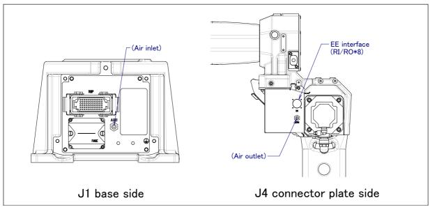
Fig. 5.3 (b) Interface for option cable (A05B-1222-H201, H231, A05B-1225-H231 are specified)
