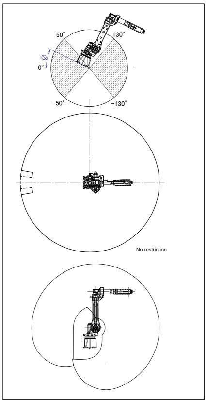
Fig. 3.6 (g) Installation area (1) operating space (M-20iA/20M) (-180° $\leq$  $\phi$  $\leq$ -130° -50° $\leq$  $\phi$  $\leq$ 50°, 130° $\leq$  $\phi$  $\leq$ 180°)
