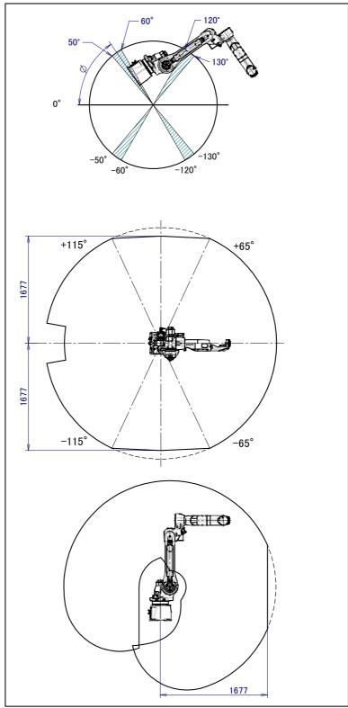
Fig. 3.6 (c) Installation area (2) operating space (ARC Mate 120iC, M-20iA)  $(-130^{\circ}\langle\phi\leq-120^{\circ}, -60^{\circ}\leq\phi<-50^{\circ}, 50^{\circ}\langle\phi\leq60^{\circ}, 120^{\circ}\leq\phi<130^{\circ})$
