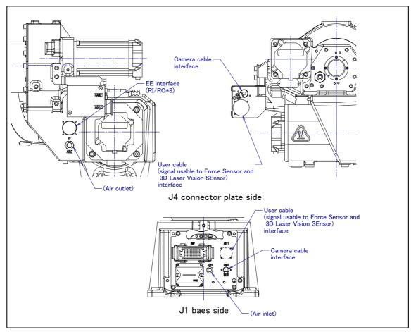
Fig. 5.3 (k) Interface for option cable (A05B-1222-H605 is specified)
