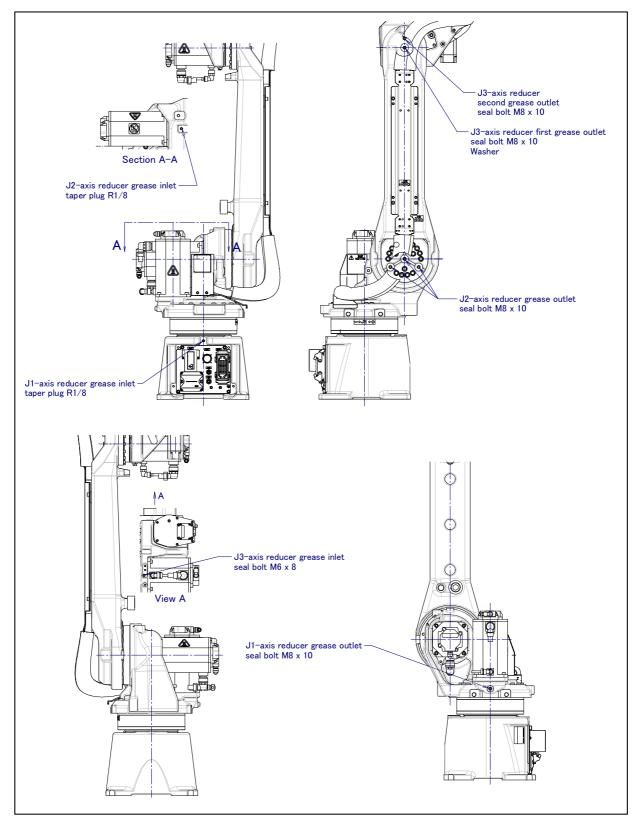
Fig. 8.3.3.1 (a) Greasing point of J1 to J3-axis reducer
