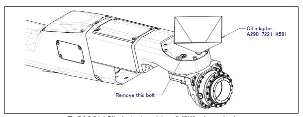
Fig.7.3.2.5 (g) Oil adapter (supplying oil J5/J6-axis gearbox) (ARC Mate 120iC/10L/12L, M-20iA/10L/12L)
