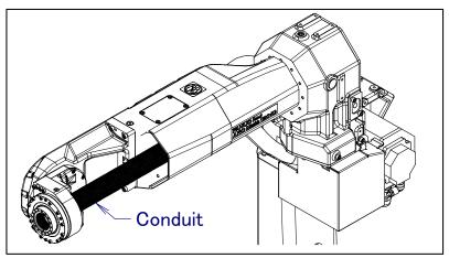
Fig. 3.4 (a) Example of "Cable integrated J3 arm"
