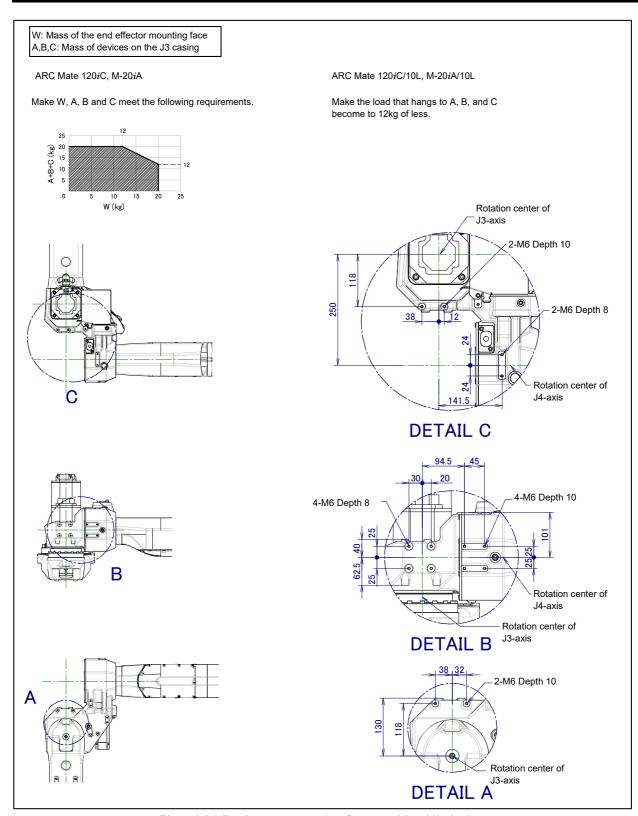
Fig. 4.2 (a) Equipment mounting faces and load limitation (ARC Mate 120*i*C, ARC Mate 120*i*C/10L, M-20*i*A, M-20*i*A/10L)
