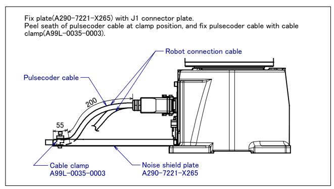
Fig.13 (a) Attaching of noise shield plate
