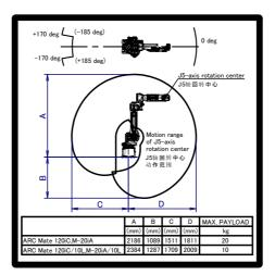
Fig. 4 (g) Operating space and payload label (Example of ARC Mate 120*i*C, M-20*i*A, ARC Mate 120*i*C/10L, M-20*i*A/10L)
