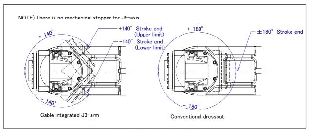
Fig. 3.3 (i) J5-axis motion limit (ARC Mate 120*i*C, M-20*i*A, ARC Mate 120*i*C/10L/12L, M-20*i*A/10L/12L)
