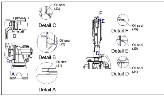
Fig. 8.2.1 (a) Check parts of oil seal
