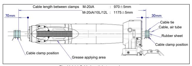
Fig. 11.1 (a) Cable length between clamps
