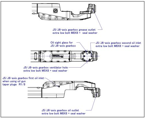
Fig. 7.3.2.5 (b) Oil inlet and outlet (ARC Mate 120iC/12L, M-20iA/12L)
