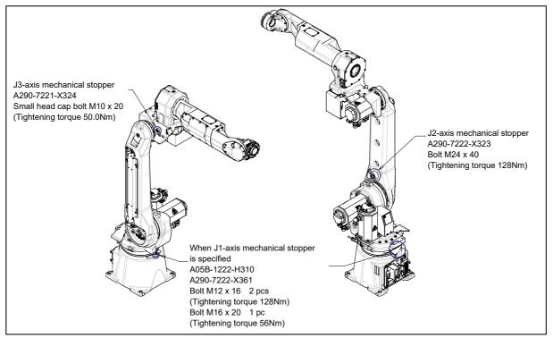
Fig. 7.2.6 (a) Check of mechanical stopper and adjustable mechanical stopper
