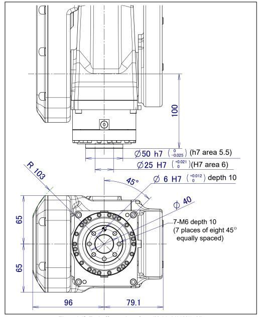
Fig. 4.1 (f) End effector interface (M-20iA/20M/35M)
