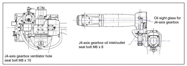
Fig. 7.3.2.3 (a) Greasing point of J4-axis gearbox (ARC Mate 120iC, ARC Mate 120iC/10L/12L, M-20iA, M-20iA/10L/12L)
