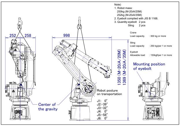
Fig. 1.1 (c) Transportation using a crane (M-20iA/20M/35M)
