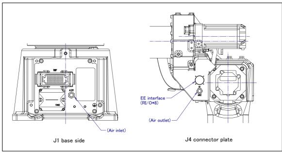
Fig. 5.3 (j) Interface for option cable (A05B-1222-H601 is specified)
