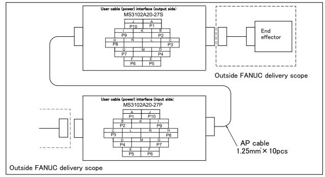
Fig. 5.3 (u) Pin layout for user cable (power line) (AP) interface (option)
