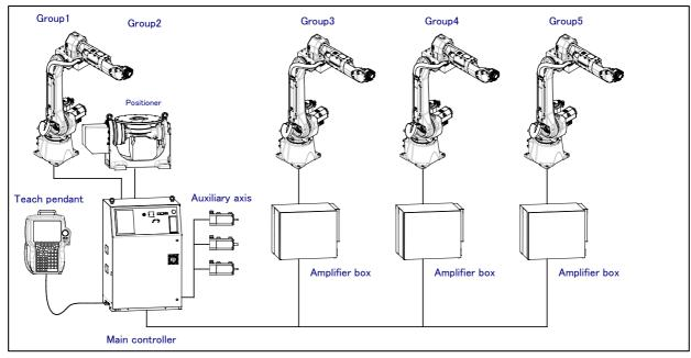
Fig. D (a) Control of multiple robots
