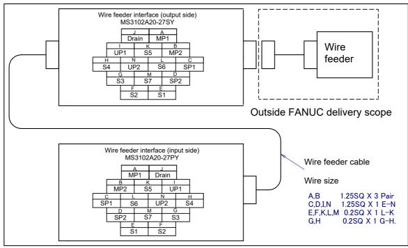
Fig. 5.3 (r) Pin layout for LINCOLN wire feeder (W/F) power supply interface (option)
