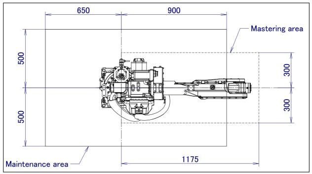
Fig. 1.3 (c) Maintenance area (M-20*i*A/20M/35M)
