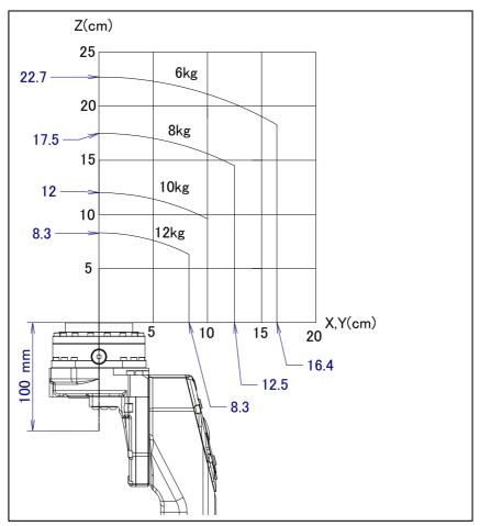
Fig. 3.5 (g) Wrist load diagram (ARC Mate 120*i*C/12L, M-20*i*A/12L 12kg wrist payload specification)
