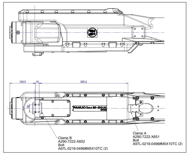
Fig. 4.2 (e) Cable clamp (option) (M-20*i*A/20M/35M)
