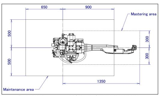
Fig. 1.3 (b) Maintenance area (ARC Mate 120*i*C/10L/12L, M-20*i*A/10L/12L)
