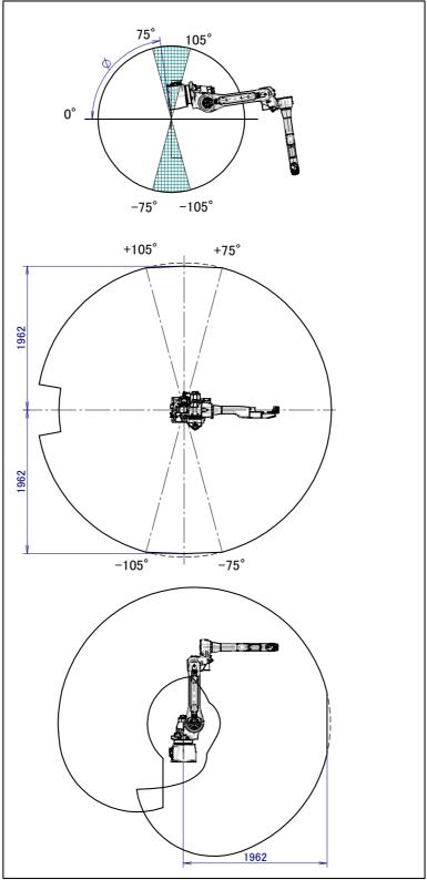
Fig. 3.6 (f) Installation area (2) operating space (ARC Mate 120*i*C/10L, M-20*i*A/10L) (-105°<φ<-75°, 75°<φ<105°)
