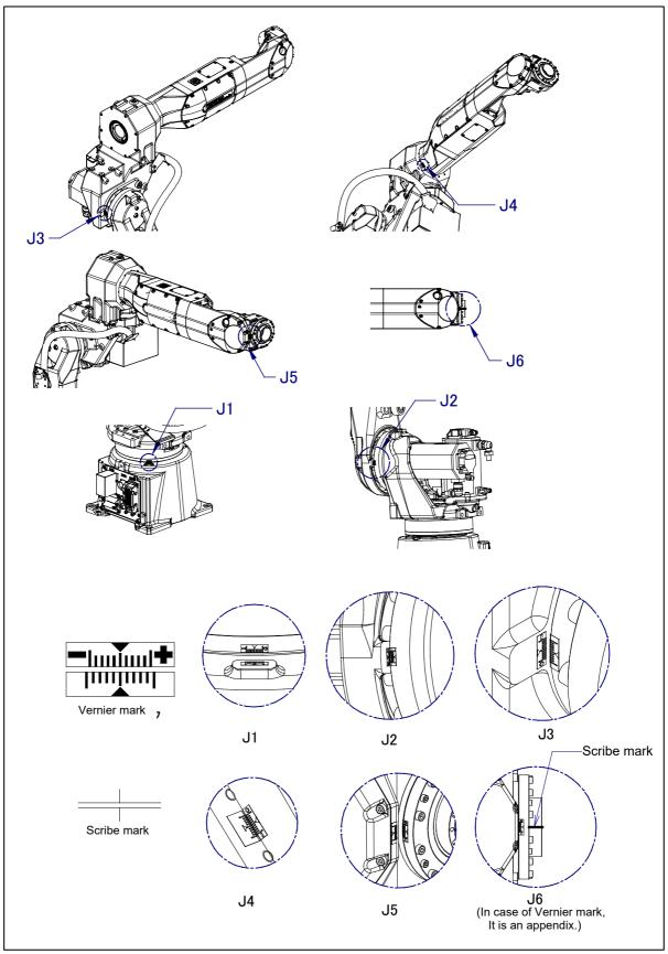
Fig. 9.3 (a) Marking position of each axis (ARC Mate 120*i*C, M-20*i*A, ARC Mate 120*i*C/10L/12L, M-20*i*A/10L/12L)
