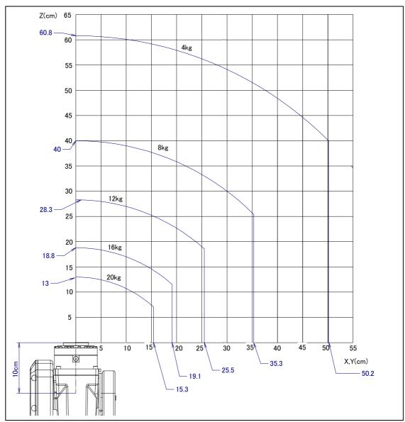
Fig. 3.5 (e) Wrist load diagram (M-20*i*A/20M)
