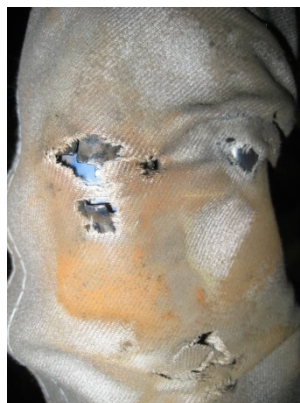
Fig. 7.2.5 (b) Damage on the cable protective sleeve
