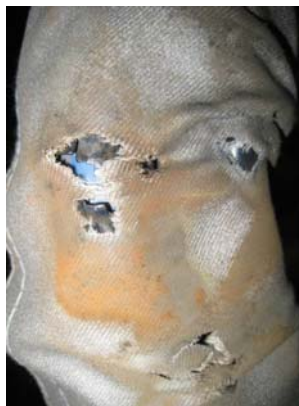
Fig. 8.2.3 (b) Damage on the cable protective sleeve
