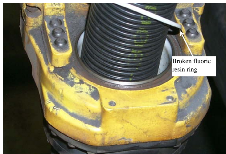
Fig .7.2.4 (b) Failure of the fluoric resin ring
