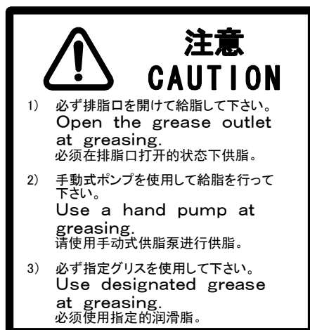
Fig. 4 (a) Greasing and degreasing label
