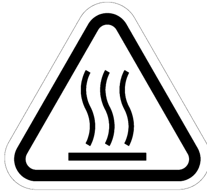
Fig. 4 (c) High-temperature warning label
