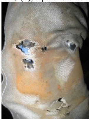
Fig. 7.2.3 (b) Damage on the cable protective sleeve
