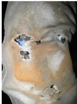
Fig. 2.2.3 (b) Damage on the cable protective sleeve
