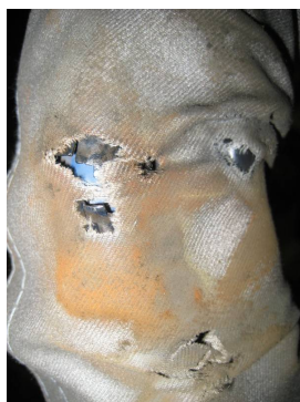
Fig. 2.2.3 (b) Damage on the cable protective sleeve
